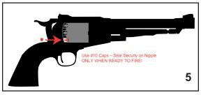
should only be tight enough so that they do not fall off the nipple when the barrel is elevated. (See Fig. 5)
