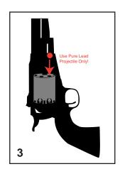
E. Grasp the rammer lever and, with a firm even stroke, seat the bullet firmly on the powder charge. (See Fig. 4) For maximum accuracy, the powder charge should be very lightly compressed by the bullet. Be sure that the bullet is seated deeply enough so that it does not interfere with the barrel and the cylinder can rotate freely. Do not leave an airspace between the powder and the bullet.
