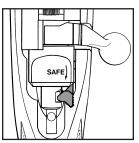
Figure 4. Safety selector in "SAFE" (full rearward) position. The safety selector is fully nested in the groove in the cocking piece. When the safety selector is in this position, the bolt handle cannot be raised. The curved arrow on the bolt sleeve indicates the direction and motion of the safety selector to bring it to the "SAFE" position. Keep the safety in this position except when actually loading, unloading, or firing.
