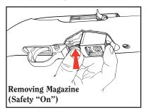
**Figure 3.** The safety should be "on" when the magazine is being removed or inserted. When the forward section of the magazine latch is pushed in (pivoted upward), the magazine is released. Depress the latch with the thumb and at the same time grasp the magazine between the thumb and forefinger and draw it out of the gun.
