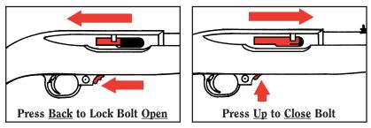
To release the bolt: Retract the bolt handle to its extreme rearward position and then press in on the <u>upper</u> section of the bolt lock. Release the bolt and it will move fully forward.
