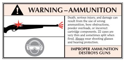
The **RUGER® MODEL 10/22® MAGNUM** is chambered for, and designed to properly function with, **only** the 22 Winchester Magnum Rimfire (22 WMR) cartridge, both jacketed and hollow point, manufactured to U.S. industry standards. Do not use any other 22 caliber ammunition in this rifle as burst cases and the release of hot powder gas can result. See "Warning – 22 Magnum Ammunition", p. 14.
