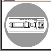
Keep the safety on unless actually firing. Always move the safety fully to its intended position and <u>check</u> it. The safety is not "ON" unless it is completely "ON". Never depend on a safety mechanism or any other mechanical device to justify careless handling or permitting the rifle to point in an unsafe direction. The only "safe" rifle is one in which the bolt is open, the chamber is empty, and there is no magazine in the gun.
