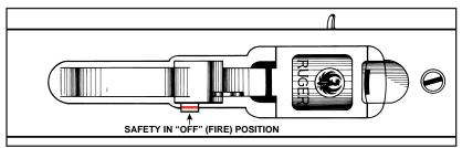
**Figure 2.** The underside of the trigger guard section of the rifle. In this illustration the safety is shown in the "off" (fire) position. The position of the safety and red band indicate the safety is "off." It should be in this position <u>only</u> when you are actually firing at a target.
