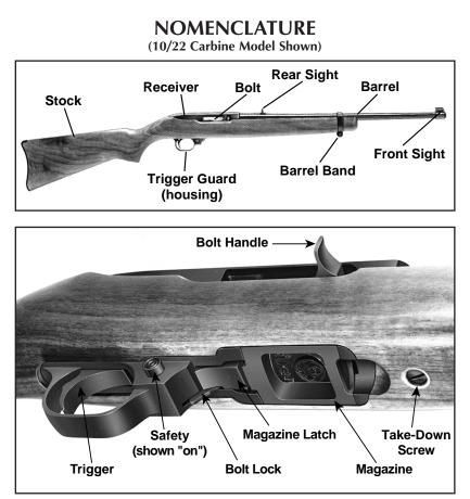
**Figure 1.** In these illustrations the frequently used operating components are identified. Note that the safety is protruding fully from the right side of the trigger guard and is therefore in its "on" (safe) position.
