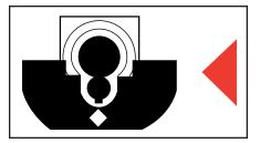
Top of front sight even with top of rear sight slide. Front sight centered in notch of rear sight slide. Target bull's-eye centered on top of front sight.
