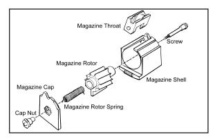
Exploded view of the 10/22 magazine components. This illustration is included to show the relationship and names of the magazine components. As noted in the text above, the magazine should not be disassembled.
