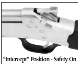
If you wish to safely decock the hammer from the fully cocked position, engage manual safety as described above and with the hammer under the full control of the user and **keeping the muzzle pointed in a safe direction**, holding and controlling the hammer with the thumb, pull the trigger and slowly and carefully let the hammer move forward until same is intercepted by the manual safety.
