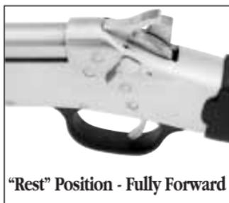
Make the Firearm Safe — The safety lever must be rotated counter-clockwise, Fully, so that the lever covers the red **F** and exposes the green **S**. THE SAFETY LEVER CAN BE ROTATED COUNTER-CLOCKWISE TO THE SAFE POSITION WHEN THE HAMMER IS IN THE REARMOST FULLY COCKED POSITION OR IS PULLED TO THE REAR ABOUT 1/2". NOTE: IN THIS POSITION, (HAMMER DOWN ON THE MANUAL SAFETY INTERCEPT), THE ACTION CAN BE OPENED AND CLOSED.
