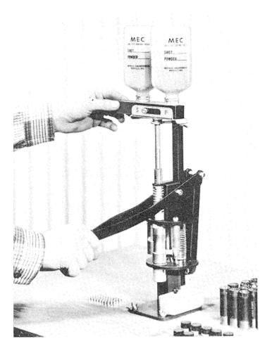
Slip shell into Resizing Die and place under Rammer Tube. Depress handle, starting Rammer Tube into shell. This operation reprimes and resizes the shell, as well as positions the "floating" wad guide. Next charge powder by pulling the charge bar to the left. (*Photo*, right).
