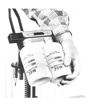
container with your hand while in the charging position so that there is no danger of its tearing loose under pressure. (Photo, right). While still supporting the shot container with your hand, flip the assembly to the upright or loading position. Now you're ready to load.
