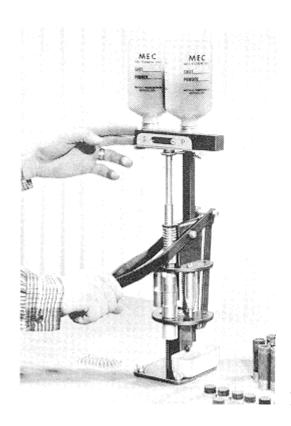
Charge shot (Photo, right) and, holding Resizing Die down, raise handle. This will allow wad guide, with Rammer Tube, to move up out of the way.
