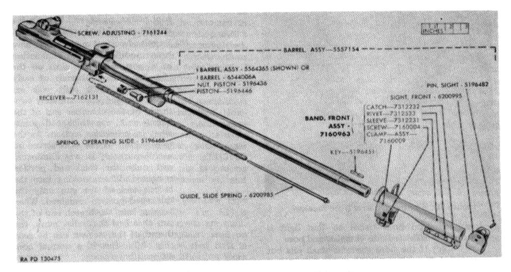
Figure 75. Barrel and receiver group M3 carbine.
