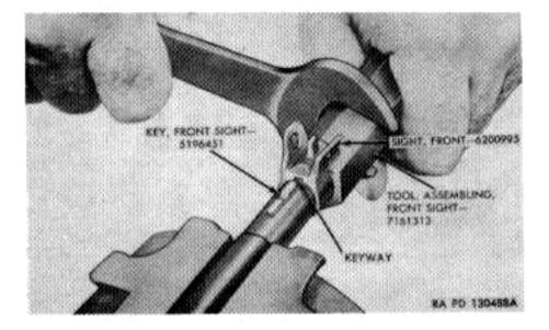
Figure 64. Aligning front sight.
