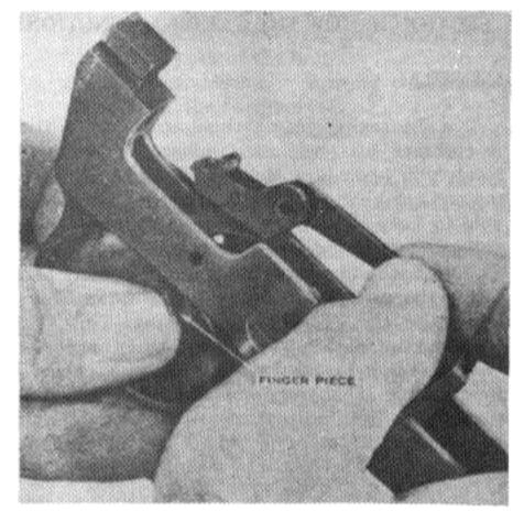
Figure 27. Replacing the trigger.
