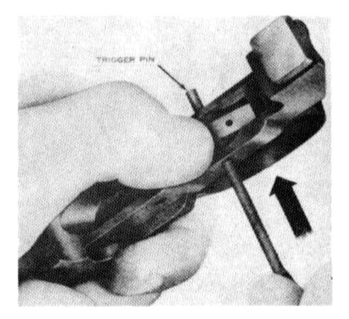
Figure 21. Removing the trigger pin.
