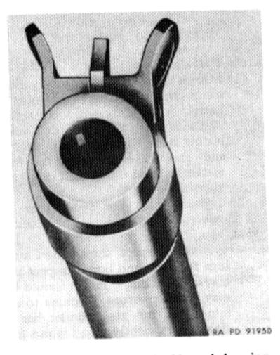
Figure 79. Muzzle end of barrel showing counterbore.
