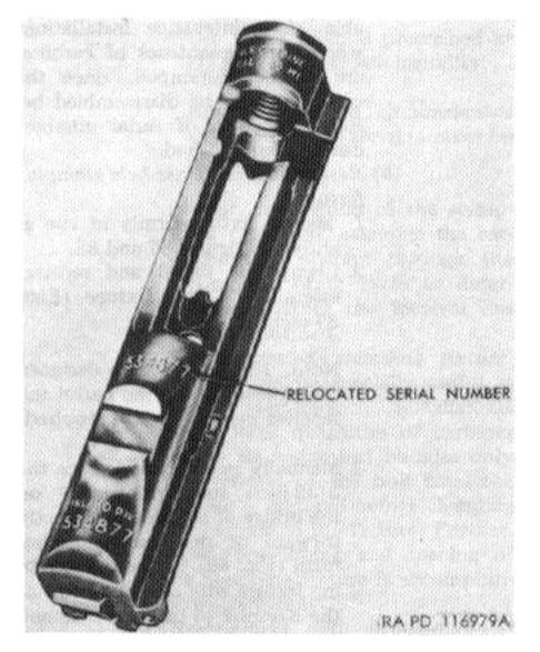
Figure 86. Relocated serial number on cal. .30 carbines.
