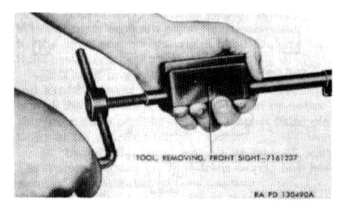
Figure 63. Removing front sight.
