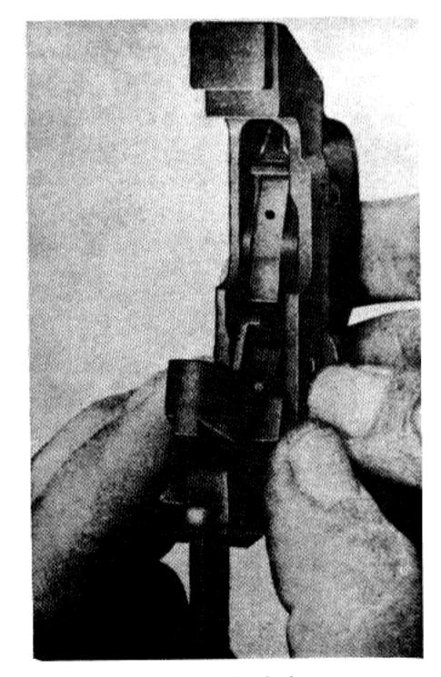
Figure 31. Replacing the hammer.
