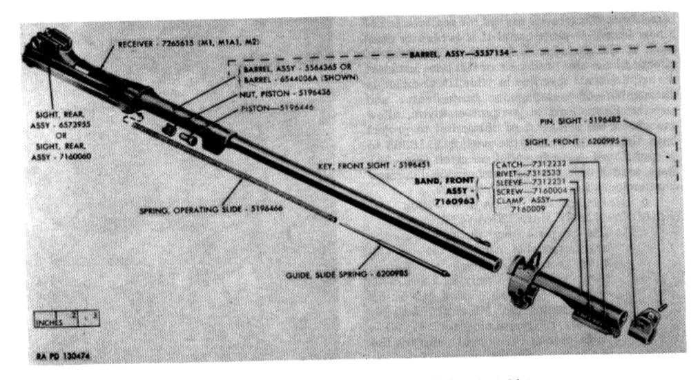
Figure 74. Barrel and receiver group M1, M1A1, M2 carbines.
