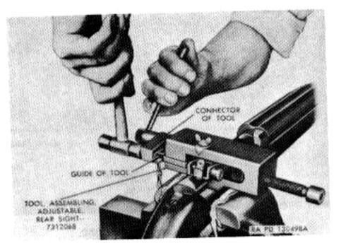
Figure 68. Removing adjustable rear sight.
