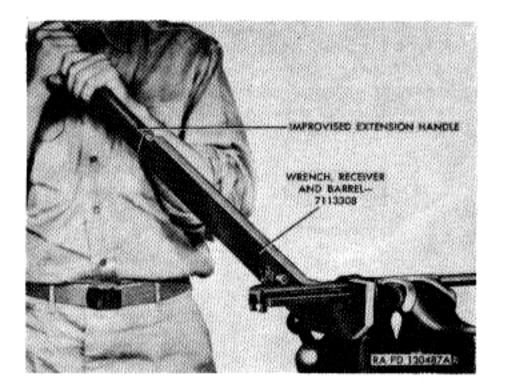
Figure 76. Removing barrel from receiver.
