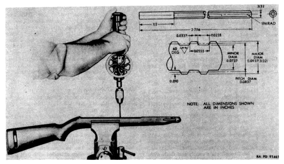
Figure 101. Installing repair screws.
