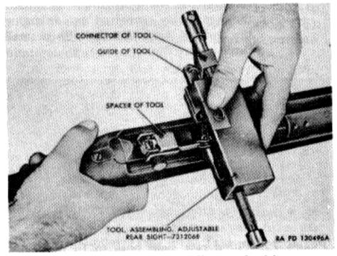
Figure 69. Rear sight assembling tool with spacer.
