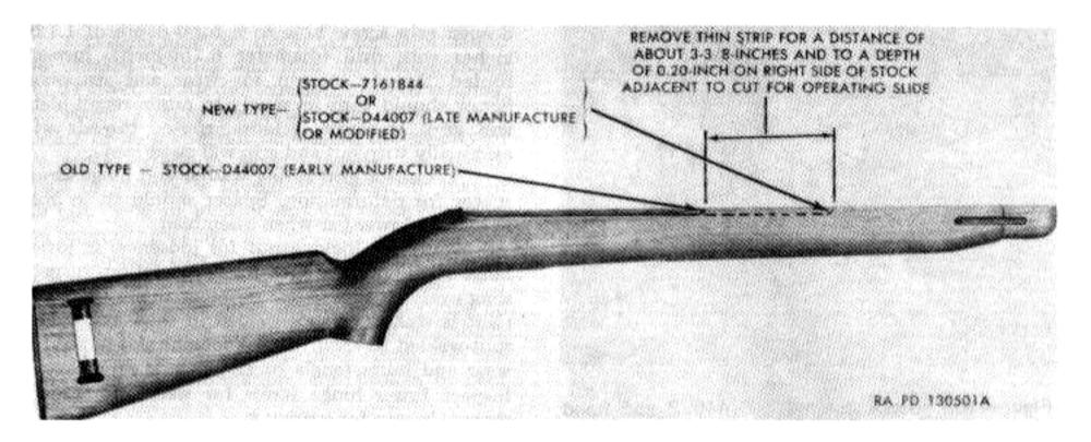
Figure 103. Modification of stock D44007 of early manufacture (carbine M1).
