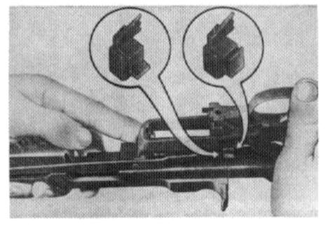
Figure 9. Removing the disconnector lever assembly.
