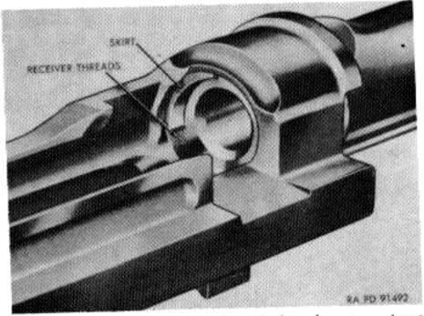
Figure 80. Breech and barrel showing new type skirt.
