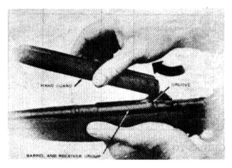
Figure 5. Removing the hand guard.
