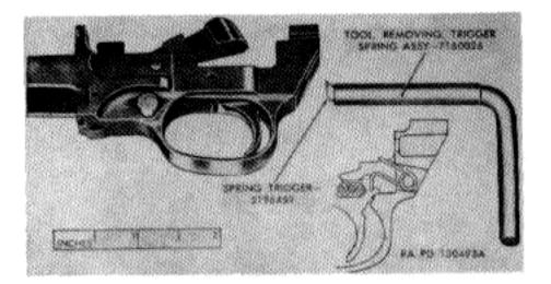
Figure 46. Trigger spring removal and installation.
