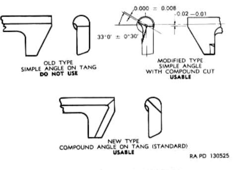
Figure 62. Firing pin 6200976.
