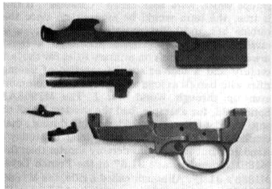
The slide, bolt, sear, magazine catch and trigger housing shown above are necessary for converting the M1 to M2 configuration, but are not considered part of the conversion kit. Not shown, and also necessary for the conversion, is the M2 stock.
