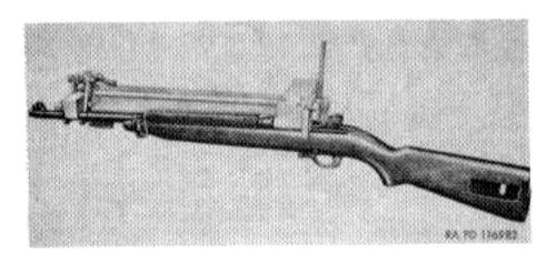
Figure 89. Carbine clamped in bench-mounted stamping fixture. able at maintenance installations where large quantities of carbines are to be restamped, since the carbines must be disassembled before relocation of serial numbers can be accomplished.
