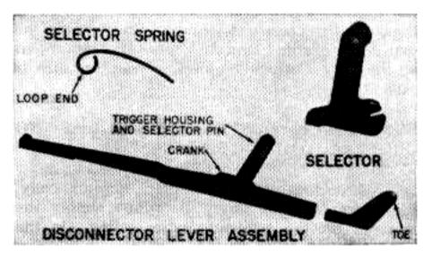
Figure 34. Trigger housing group parts.
