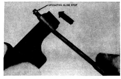
Figure 32. Removing the operating slide stop.
