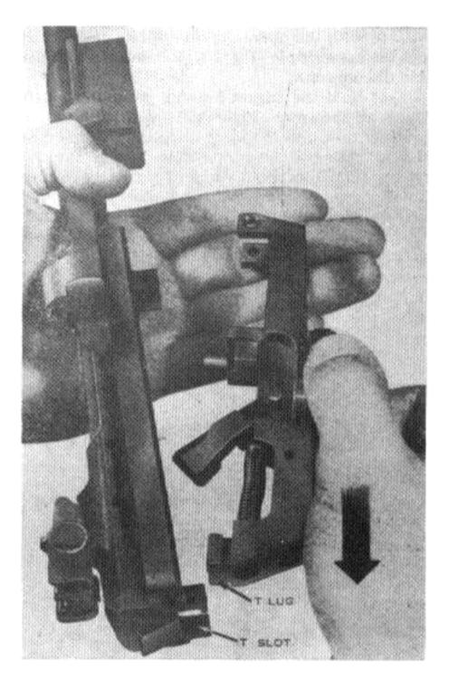
Figure 16. Replacing the trigger housing group.
