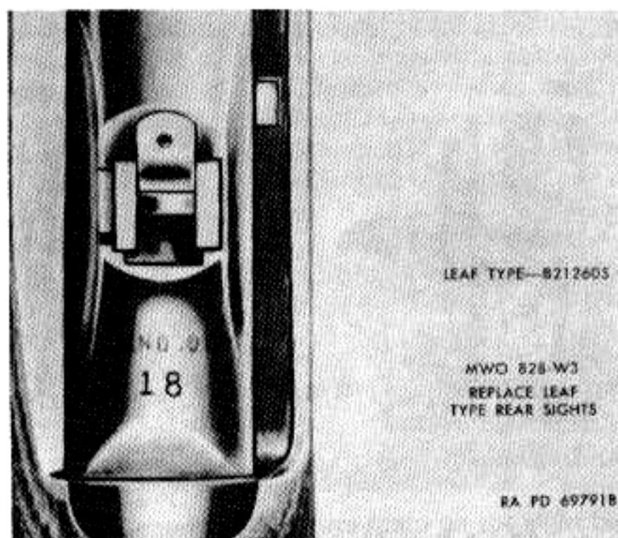
Figure 66. L-type (leaf type) rear sight assembly.
