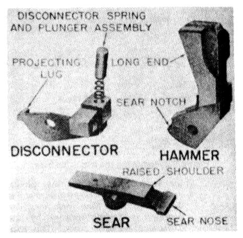
Figure 35. Trigger housing group parts.
