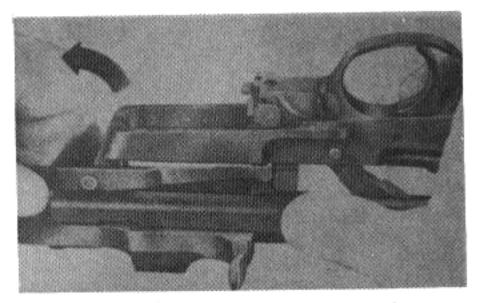
Figure 10. Removing the disconnector lever assembly.
