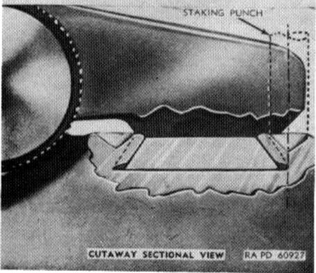
Figure 73. Rear sight showing staking.
