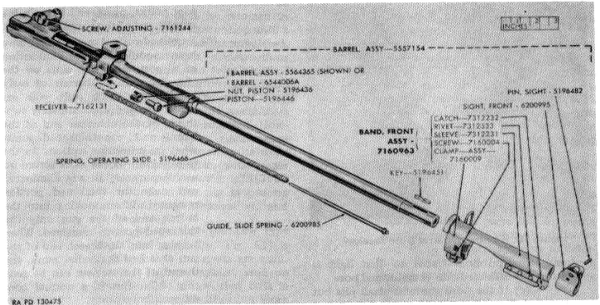
Figure 75. Barrel and receiver group M3 carbine.
