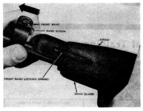
Figure 4. Sliding the front band forward.
