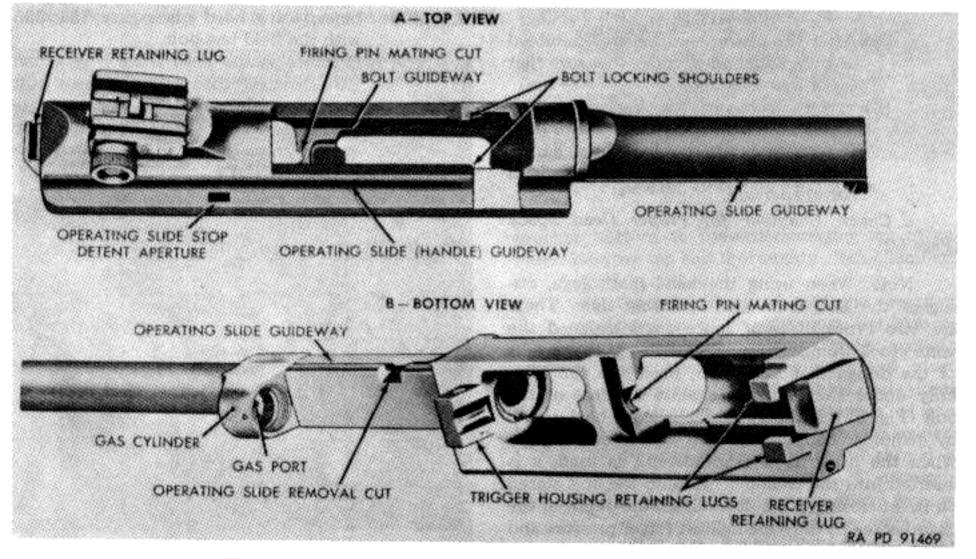
Figure 78. Barrel and receiver group - points of inspection.
