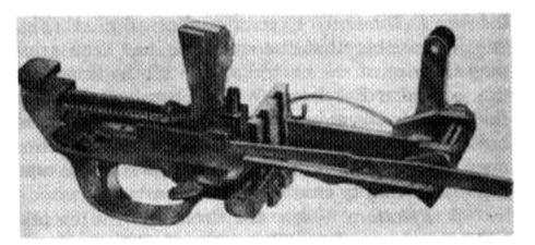
Figure 38. Functioning of trigger housing group.
