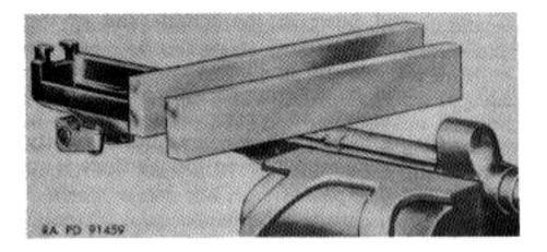
Figure 92. Checking barrel and receiver alignment.
