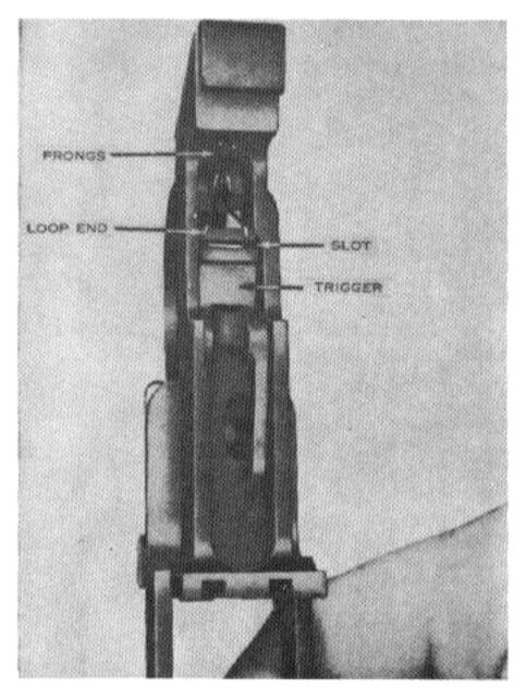
Figure 28. Trigger spring in proper position.
