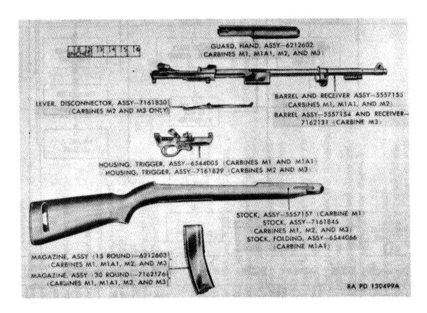
Figure 43d. Assemblies comprising the weapon shown in relative positions.
