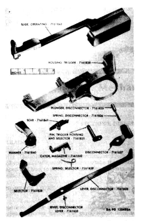
Figure 3b. Operating parts for carbines M2 and M3.
