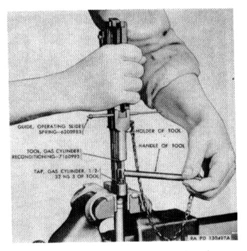
Figure 83. Chasing gas cylinder thread.
