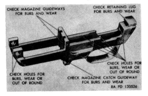
Figure 47. Trigger housing inspection points.
