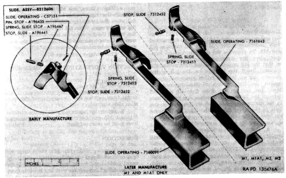
Figure 57. Operating slide assembly.
