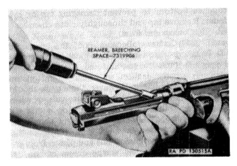
Figure 84. Reaming chamber for head space.
