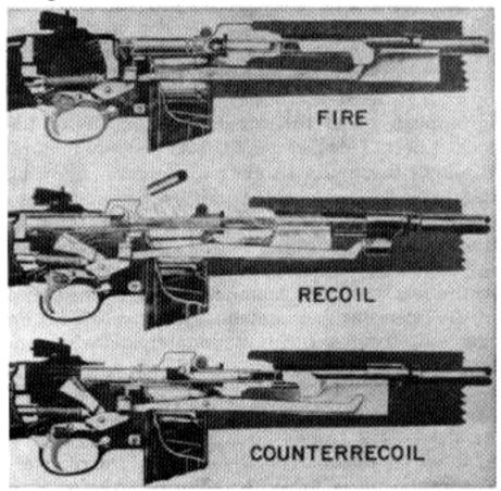
Figure 39. Functioning of operating parts (semiautomatic setting).
