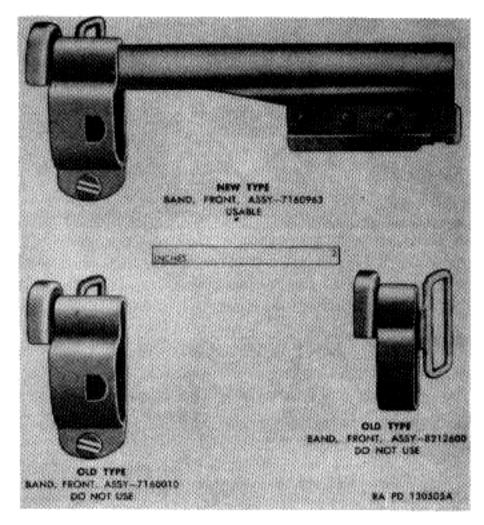
Figure 81. Front band assemblies.
