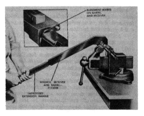
Figure 91. Assembling barrel to receiver.
