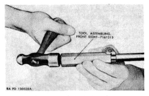
Figure 65. Installing front sight.
