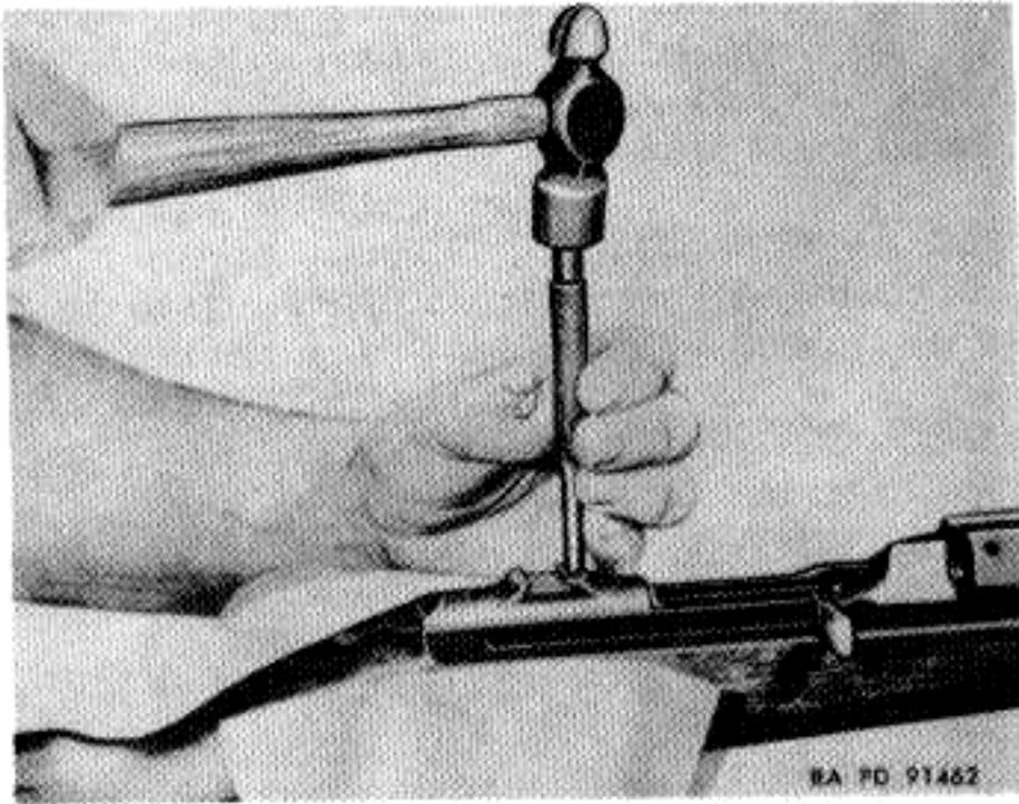
Figure 71. Peening receiver to reduce oversize dovetail slot.
