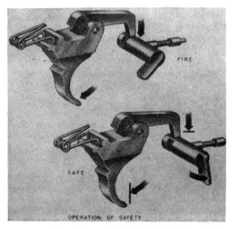
Figure 43. How the safety works.
