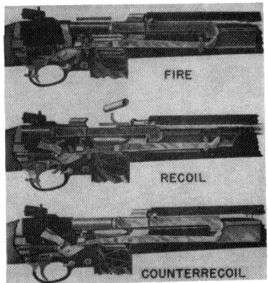
Figure 42. Functioning of operating parts (automatic setting).
