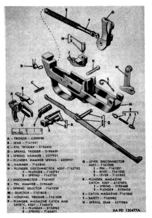
Figure 56. Trigger housing group - carbines M2 and M3.
