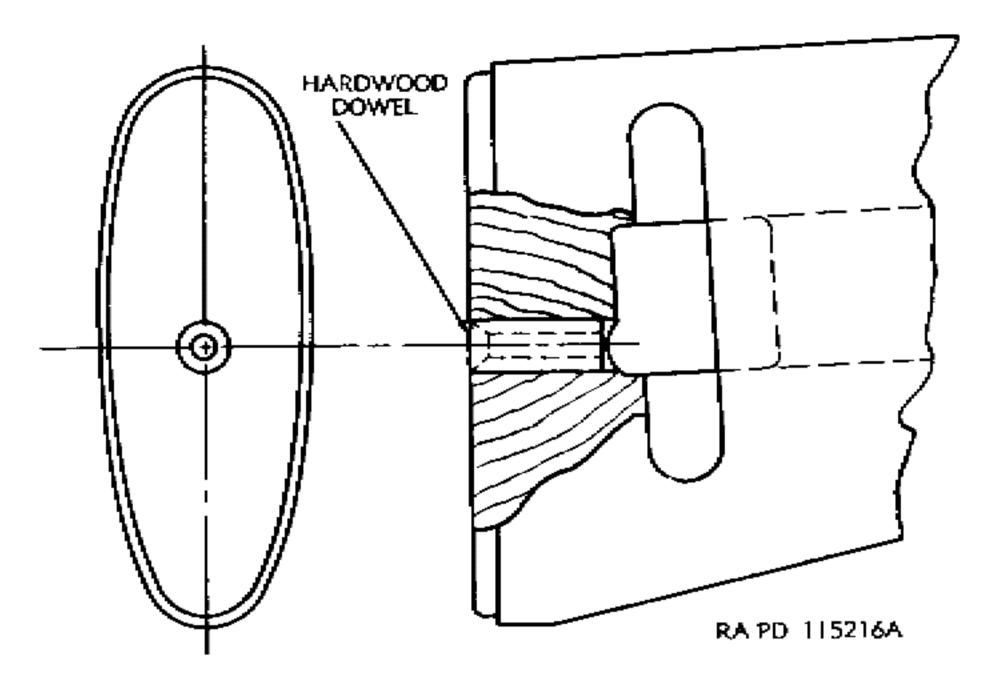
Figure 102. Repair for stripped screw hole.
