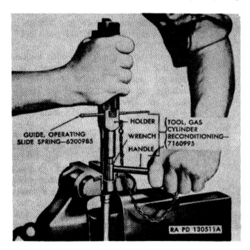
Figure 77. Removing piston nut from gas cylinder.
