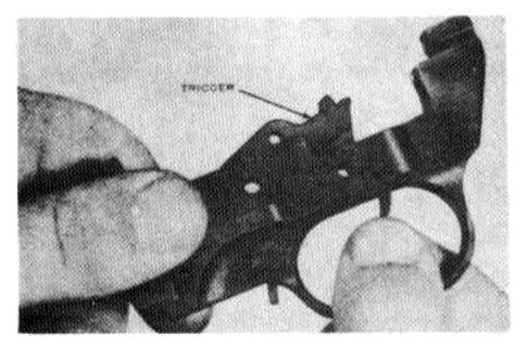
Figure 22. Removing the trigger.
