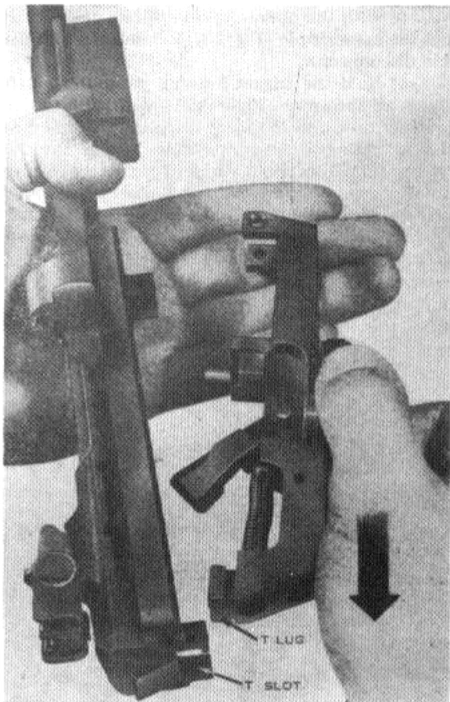
Figure 16. Replacing the trigger housing group.
