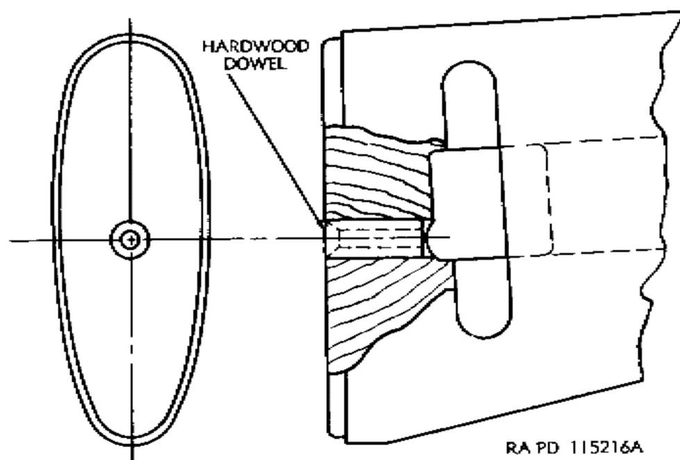
Figure 102. Repair for stripped screw hole.
