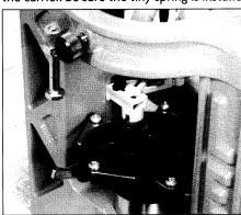
into the hole at the rear of the primer punc Now slip the primer trough over the punch Push down on the left end of the priming rocker arm to be sure everything is working freely. The primer punch will be seen moving up as you push down on the priming rocker arm.
