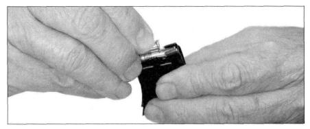
and insert it into the bottom of the floor plate in front of the trigger guard. The magazine catch should click into a locked position even with the bolt closed.
