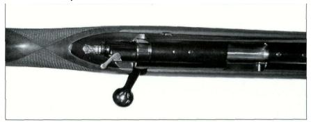
When you are ready to fire push the serrated lever fully to the forward position. The safety mechanism is fitted into position before the rifle leaves the factory. You should see a red dot on the back of the safety.
