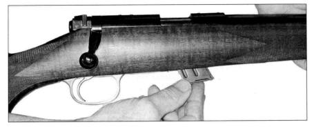
By recycling the bolt backwards and forwards, loaded rounds should enter into the chamber in a controlled manner. In other words, the rim of the cartridge case should slide up into the bolt face as the bolt is moved forward and cartridges picked up out of the magazine. The cartridge will then feed into the chamber. The bullet should not touch any part of the mechanism as it is feeding into the chamber.
