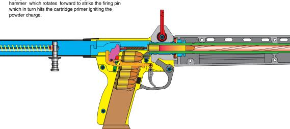
After about 3/16 (5 mm) of bolt travel (or .0013 seconds) the bullet exits the muzzle. The pressure in the barrel has now dropped to a low level.
