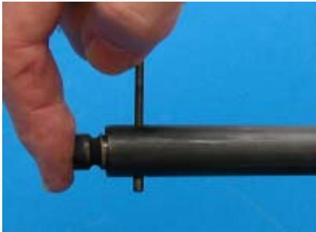
now be able to be pulled straight out of the bolt carrier. After the operating handle is removed the bolt carrier assembly can now be guided out of the bottom of the receiver by holding onto the recoil spring tube.
