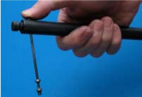
now free to be taken off. Slide the recoil spring tube off the piston rod and remove the recoil spring from the recoil spring tube.
