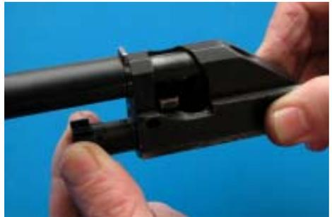
spring tube so that the locking tab points towards the top of the bolt carrier. Check the operation of the recoil spring by lightly pulling on the recoil spring tube to compress the spring.
