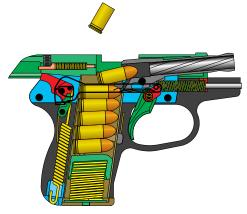
During the rear recoil motion, the hammer is disengaged and follows the slide acting like an extra recoil spring. As the slide moves forward, the hammer rotates with it until the hammer block reengages the hammer holding it away from the firing pin. When the trigger is released the trigger bar moves backwards and behind the hammer catch. The P-3AT is then ready for the next shot.
