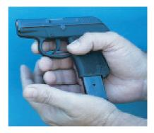
Hold the pistol in one hand with the muzzle pointing in a safe direction and with your finger off the trigger and outside the trigger guard. Insert the loaded magazine into the grip until it is locked in place. Check to assure magazine is secure. Pull the slide back and release. This strips a round from the magazine and seats it in the barrel chamber. At all times keep your hands away from the muzzle.
