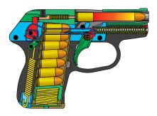
Close to the rear position, the empty case hits the ejector, and is thrown out of the gun. The recoil springs drive the slide forward again. The top cartridge in the magazine is picked up by the breech face and pushed into the barrel. Close to battery the barrel is cammed up, positively locking into the slide.
