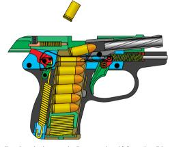
During the rear recoil motion, the hammer is disengaged and follows the slide acting like an extra recoil spring. As the slide moves forward, the hammer rotates with it until the hammer block reengages the hammer holding it away from the firing pin. When the trigger is released the trigger bar moves backwards and behind the hammer catch. The P-32 is then ready for the next shot.
