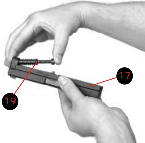
8. Remove the barrel (18) from the slide (17).
