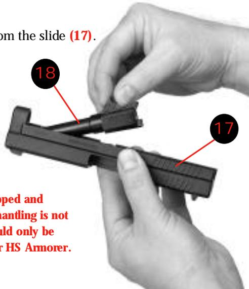
**The pistol is now fully field stripped and ready for cleaning. Further dismantling is not necessary for cleaning and should only be done by a qualified gunsmith or HS Armorer.**
