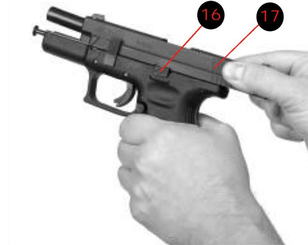
6. Now slip the complete assembly {slide (17), barrel (18) and dual tension recoil spring (19)} forward and off the frame (20).
