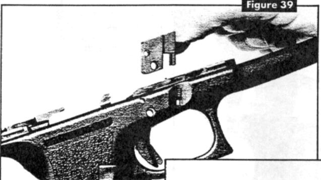
Then remove the locking block by hand (Figure 39).
