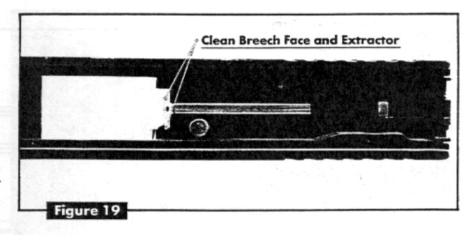
slide, and possibly contribute to malfunctions of the pistol. The pistol should be field-stripped every time it is cleaned.
