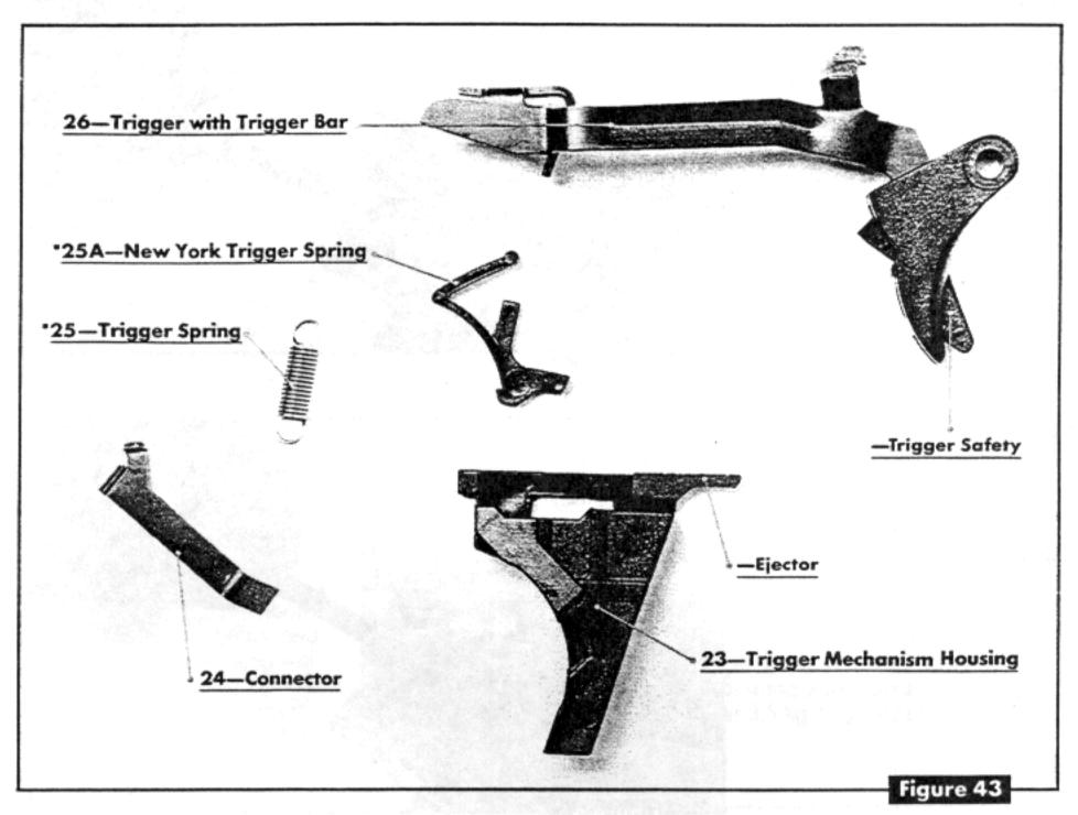
\*Either the standard trigger spring or the New York Trigger Spring can be used.
