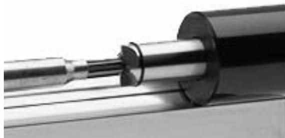
The Forster Neck Reamer will remove excess brass from the inside neck walls of cartridge cases. High-grade tool steel and a staggered-tooth design enable the Forster Neck Reamer to cut brass smoothly without chatter. Forster Neck Reamers are ground .0025"-.003" larger than maximum bullet diameter, therefore **neck reaming should be done after the case has been fired with a full load and before the neck or full length sizing operation.**
