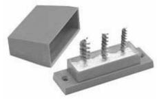
Fasten the base of the Graphiter to a loading bench or block of wood for stability. Level off graphite powder in the base of the Case Graphiter. Slide the empty case up and down on the proper-sized brush (the three brushes will accommodate all popular calibers). This cleans and lubricates the case neck. Replace the cover when the Graphiter is not in use. Wipe the white mica (graphite) off the outside diameter of the case necks to prevent scratching during the sizing process.
