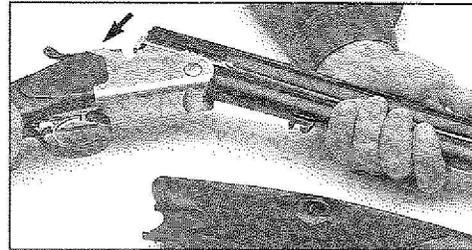
(figure 3) Barrels being placed on receiver group
