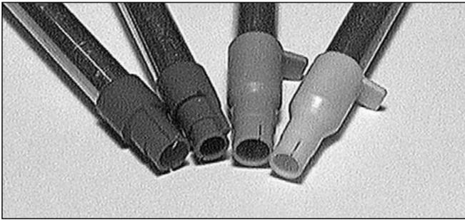
**Fig. 14** - The machine comes with two primer pickup tubes (#20060 Lg, #20059 Sm) and two primer magazine tubes (#22031 Lg, #22030 Sm). Each has a large and small. They are color coded for easier identification. See page 13 for color coding information. The large ones should be used together and the small ones should be used together. You will notice that the primer magazine tips have an indexing ridge to assist in their placement in the primer feed system.
