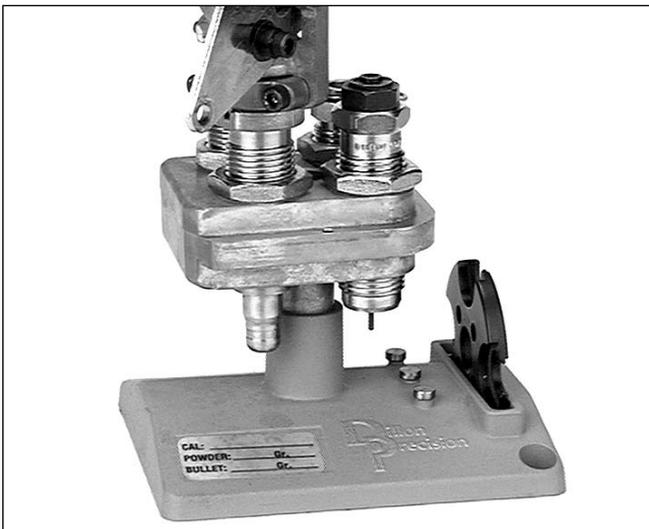
**Fig. 15** - A complete, removable toolhead with all of the dies adjusted. Toolhead stand is optional.
