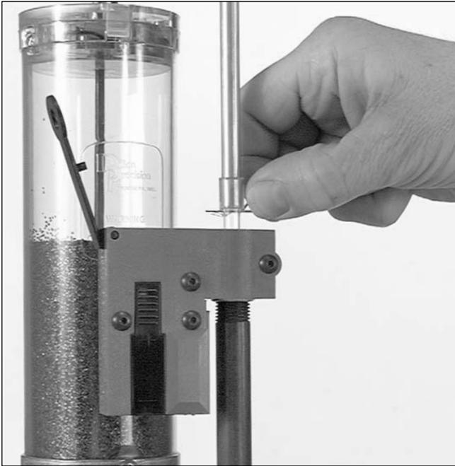
**Fig. 25 - Drop the primers into the primer magazine.**
