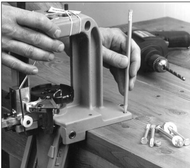
**Fig. 1 - Using the machine as a template, mark and drill four 1/4 inch holes allowing 12 inches on each side for your work area.**
