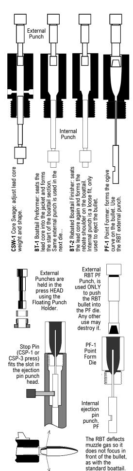
Never try to swage a component that will not go into the die by hand. The swaging operation depends on each component being slightly smaller than the die bore, and increases the bullet diameter a little with every step. The core seating die and point forming die are matched to each other for a given jacket and core material to within 0.0005 to .0010 inches with the core seater being smaller.
