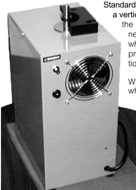
The PCM-1 rolls precise cannellure in bullets, and other straight-sided cylinders, made of copper, brass, aluminum or mild steel tubing with walls up to .050-inches thick. It is not recommended for rolling cannellure in solid rod, and is not warranted for such use. Solid copper, brass, aluminum or steel bullets, or other designs having the same resistance to compression, may cause damage to the main thrust bearing or motor, or produce accelerated wear.
