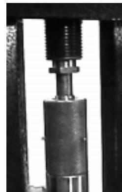
The LSWC-1 die is used to make all-lead, gas-checked, or Base-Guard™ bullets which have a semi-wadcutter shoulder between the ogive and the shank. The nose is formed in a cavity, machined in the external punch (although the base and nose can be formed in the alternate punches if requested) with the base being formed against the face of the internal punch.
