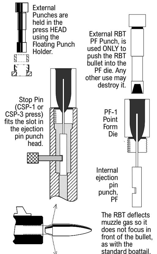
Never try to swage a component that will not go into the die by hand. The swaging operation depends on each component being slightly smaller than the die bore, and increases the bullet diameter a little with every step. The core seating die and point forming die are matched to each other for a given jacket and core material to within 0.0005 to .0010 inches with the core seater being smaller.
