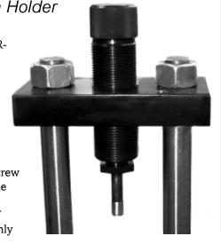
press head, replacing the punch holder, and have their own punches which screw into the 1-inch by 12 turn/in threaded ram of the press. The punch for a drawing die faces upward, pushing the component through the bottom of the die and out the top. The punch for a swaging die hangs down from the punch holder, facing the ram and the die screws into the ram, facing up. Swage dies eject the bullets from the top, the same direction in which they are inserted.
