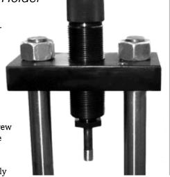
press head, replacing the punch holder, and have their own punches which screw into the 1-inch by 12 turn/in threaded ram of the press. The punch for a drawing die faces upward, pushing the component through the bottom of the die and out the top. The punch for a swaging die hangs down from the punch holder, facing the ram and the die screws into the ram, facing up. Swage dies eject the bullets from the top, the same direction in which they are inserted.
