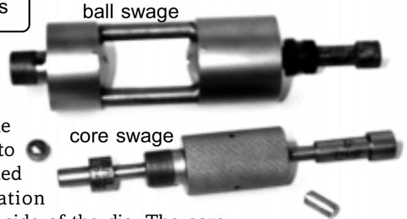
1) Swage the cores to the indicated core weight, above, using the core swage die. The lead cores can be cast, or cut from lead wire to a weight that is from 3 to 5 grains more, and the surplus lead is bled
