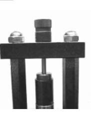
Bullets can usually be reduced at least 0.005-in diameter, depending on the material strength and thickness of the jacket walls. It is possible to reduce .357 pistol
