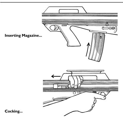
Place left hand in the space between the carry handle and slide rearward as far as possible. When the furthermost point of this motion is reached, remove hand to allow the cocking handle to slide forward. The cocking handle will automatically return to its previous position to form part of the carry handle.
