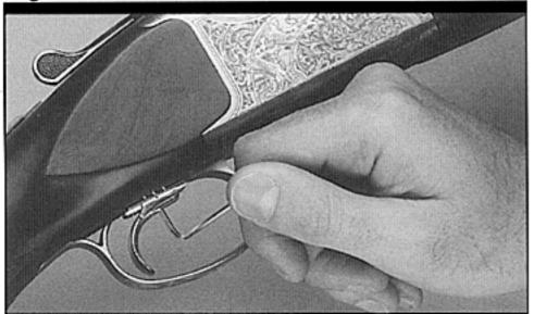
Wipe all metal surfaces off the receiver, forearm and barrels with a clean rag. Then lightly oil your gun at the points described in step 2 under "Assembly" on page 6. Regular, light oiling is extremely important to the durability and reliable operation of your shotgun.
