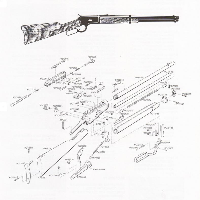
Schematic is provided for parts identification only and should not be used as a guide to assemble guns.
