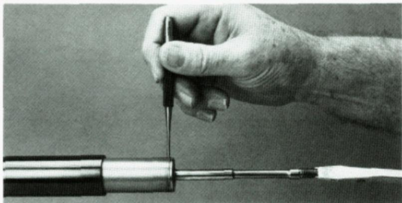
Remove the punch and continue turning the magazine retainer and forearm cap stud until three threads are exposed. At this point lay the screwdriver aside and proceed by hand. (See Figure 28.)
