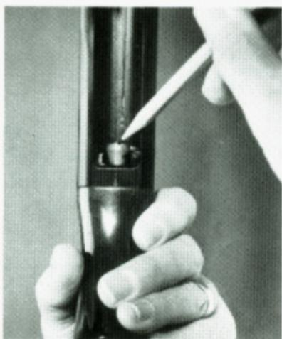
will go all the way back before continuing assembly. If the bolt will not go back freely, remove the assembly and align all components carefully, then repeat procedure.
