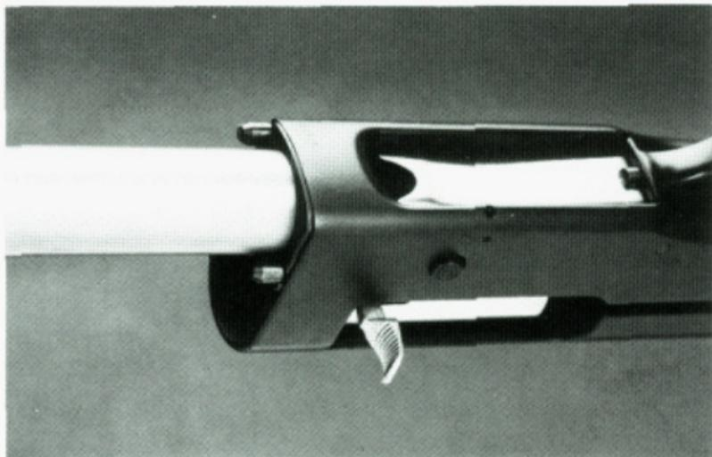
Replace the forearm and forearm cap assembly. If there has been no recoil adapter installed, and your individual gun will not function reliably with light target loads, you should proceed with the following:
