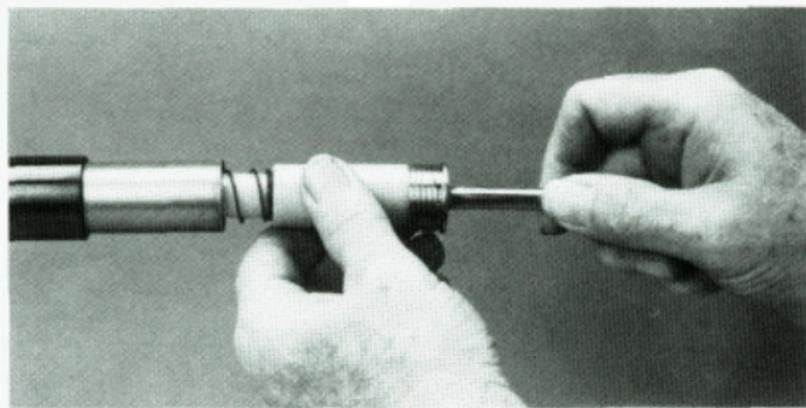
**NOTE:** The magazine plug is spring loaded and under tension. Be prepared to use both hands in guiding the spring out of, and back into, the magazine tube once the plug has been removed.
