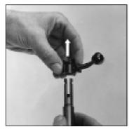
• Then remove the bolt handle assembly.
