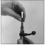
• Now remove the firing pin assembly.
