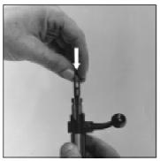
Replace the firing pin assembly and make sure that the lug lines up with the longer slot in the bolt body and the bottom of the recess at the bolt handle as shown.
