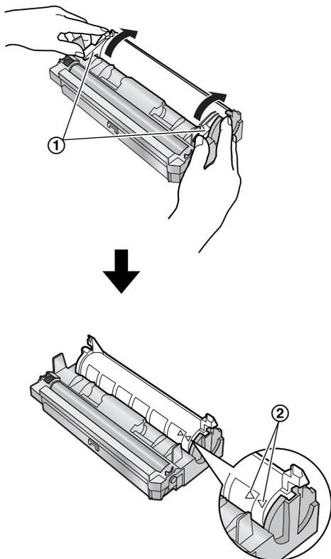
6 Remove the used cartridge (①) from the drum unit (②).
