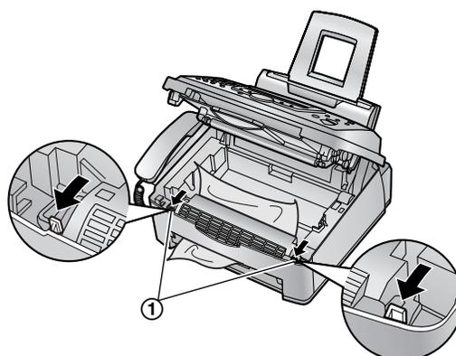
3. Remove the jammed paper (①) from the fuser unit by pulling it upwards carefully, then install the drum and toner unit.
