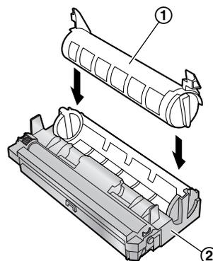
8 Firmly press down the toner cartridge to snap into position (①).
