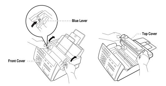
4 Pull the jammed paper gently from the paper feeder toward the back of the fax machine. If the paper remains jammed, then pull it toward the front of the machine.
