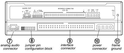
**7** analog audio output connector: You can use an audio cable to connect this connector to the audio input connector on a sound card. Pin assignments are described below:
