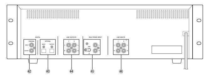
The CC-222MKII line analog inputs and outputs all operate at the -10dBV level. For details of input and
