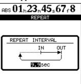
**2** Use the wheel to set the interval, and ENTER to confirm the value.
