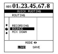
**1** Press the QUICK ROUTING key to bring up the screen shown here.
