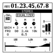
**3** Use the cursor keys and wheel to select and adjust the EQ parameters for the stereo bus.
