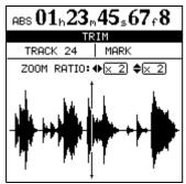
**3** Press the SELECT key of the track that you want to view. The display changes to the waveform of that track.
