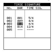
**2** This is very similar to the tempo map. Use the INSERT and DELETE keys to insert and delete entries and the cursor keys to scroll through the list.
