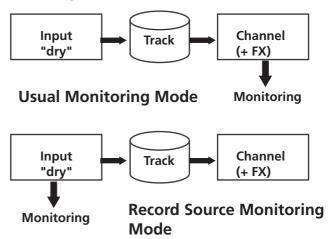
In the record source monitor mode, the source is the input.
