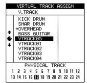
2 Use the channel SELECT keys or the ( ◄ and ► keys) to select the disk track to which the virtual track will be assigned, as shown by the inverted numbers at the bottom of the screen.
