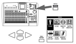
Use the cursor keys to move around the screen, and press **ENTER** when the function you want to use is highlighted.
