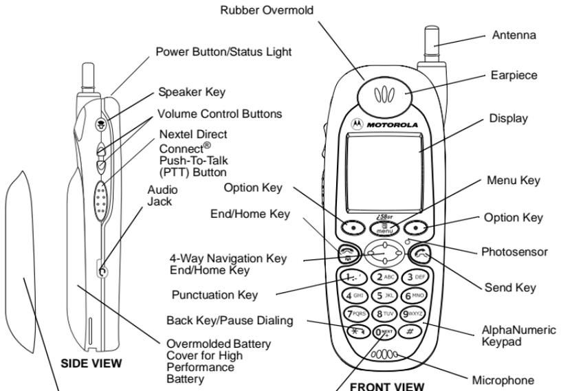
Overmolded Battery Cover for Maximum Capacity Battery
