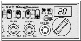
While holding mic button adjust the SWR CAL knob so the meter needle swings to the CAL ▼ mark on
