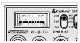
• The S/RF-SWR-CAL switch must be in the S/RF position to read the meter.
