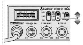
• When switched to ANL the Automatic Noise Limiter is activated. This helps reduce noise created by the vehicle's electronics.
