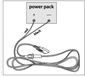
1 Simply connect the red (+) and black (-) leads of the transceiver to the corresponding terminals of the power pack.
