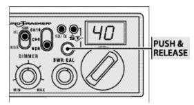
Push and release the ST button. Red LED is illuminated when SoundTracker™ is turned on.
