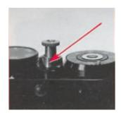
With the finger tip depress the Film Rewind Sleeve (arrowed above) into the cut-out portion of the surrounding sleeve. It will click and stay down.
