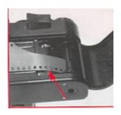
[22] slots ensuring that the second hole engages with a tooth on the spool. Ease film forward by swat strokes of Transport Lever [2] until it stops. The lower Sprocket Teeth [26] should be properly engaged.
