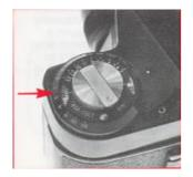
Set the speed of the film in use by turning the dial with the small projection. Any intermediate positions may be used and are proportionate
