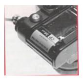
Insert film cassette into Film Chamber [21] projection of cassette to bottom.
