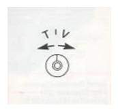
Make sure that the indicator on the Shutter Release Button [3] is facing towards the front of the camera.
