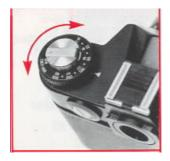
Set Film Speed Selector Dial [15] against Indicator [17] appropriate to the speed of the film to be used. There are two scales for films rated in ASA and DIN. Only click-stopped numbered or intermediate positions may be used. Intermediate positions are proportional. If using 1000 ASA film set the selector to 500 ASA but use the next faster shutter speed than indicated by the meter or close the aperture ring by one full stop.
