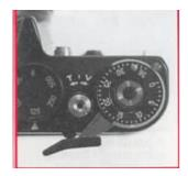
Depress Shutter Release button [3] halfway until lens closes down and turn it fully clockwise to the "V" position.
