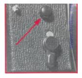
Press the Self-Timer Release Button p1 and move into the picture area as quickly as possible. The Lever [8] will slowly return firing the shutter during its travel.
