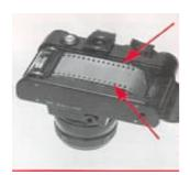
Fire shutter. Advance film by short strokes of transport lever until both top and bottom sprockets are engaged. If necessary tighten film on Take-up Spool [22] by turning the flange at the base of the spool anti-clockwise with the finger and in the cassette by gently turning the Rewind Knob [16] in the direction of the arrow on the lever until resistance is felt. This is especially necessary with twelve exposure films.
