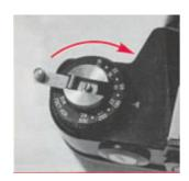
Lift out Rewind Crank [16] and rotate clockwise in the direction of the arrow. You will feel the film being rewound into the cassette - stop when resistance ceases.
