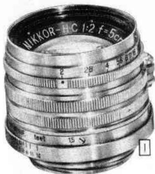
All NIKKOR lenses are coated on the inside only. It is believed the coating of inside surface only will help prevent scratches. It is evident that if the front element or outside of the lens were coated, this coating would be more subject to scratches than the hard, uncoated outside surface. The coating can be recognized in ordinary light by its reddish-to-blue cast. This coating is fused to
