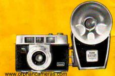
The Kodak Generator Flasholder, Type 1, is a small, compact, pocket-sized flasholder which uses no batteries. A spin of the generator handwheel charges the capacitor with ample power to fire the flash lamp. The flasholder accepts No. 5, No. 25, M5, M25 or M2 bulbs.
