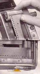
Insert the film magazine in the recess next to the knob. Push the rewind knob all the way in, turning it slightly if necessary.
