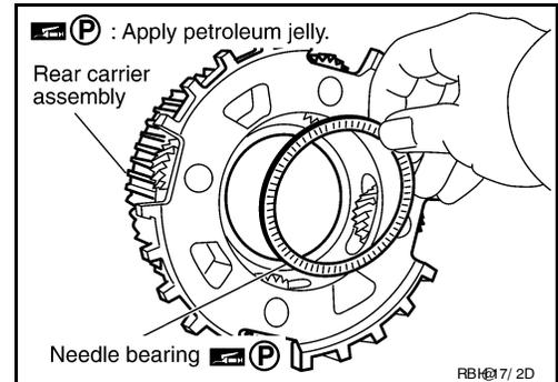
41. Install bearing race in rear carrier assembly.
