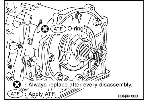
6. Remove oil pump assembly to transmission case bolts.
