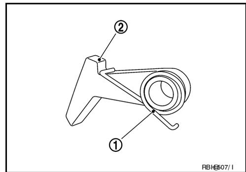
27. Install parking pawl (with return spring) and pawl shaft to rear extension (2WD models) or adapter case (4WD models).
