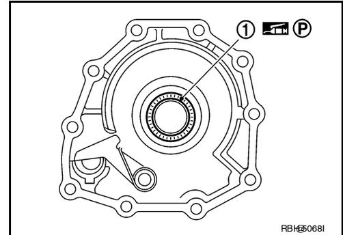
30. Install seal rings to output shaft.
