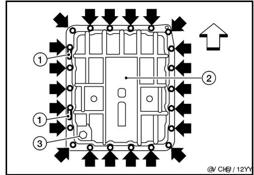
3. Tighten oil pan bolts in numerical order as shown.
