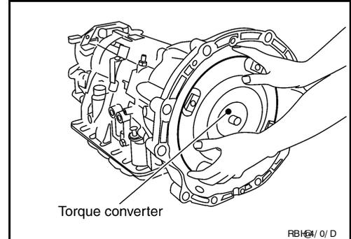
3. Check torque converter one-way clutch using a check tool as shown.
