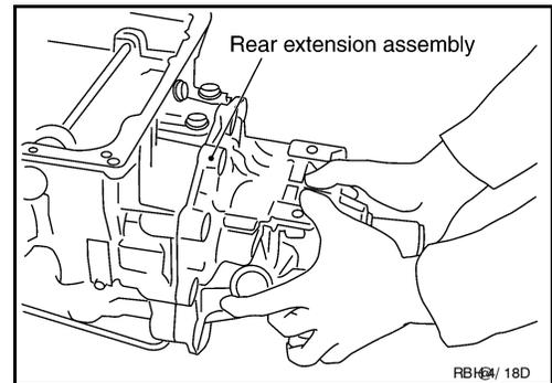
iii. Install the rear extension assembly bolts and tighten to the specified torque.
