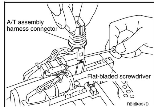
18. Disconnect TCM connector and park/neutral position switch connector
