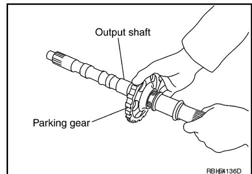
32. Install output shaft in transmission case.
