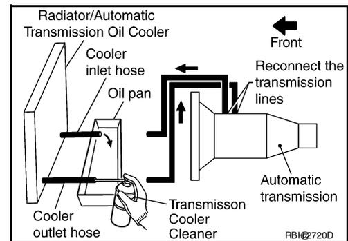
7. Insert the tip of an air gun into the end of the cooler outlet hose.
