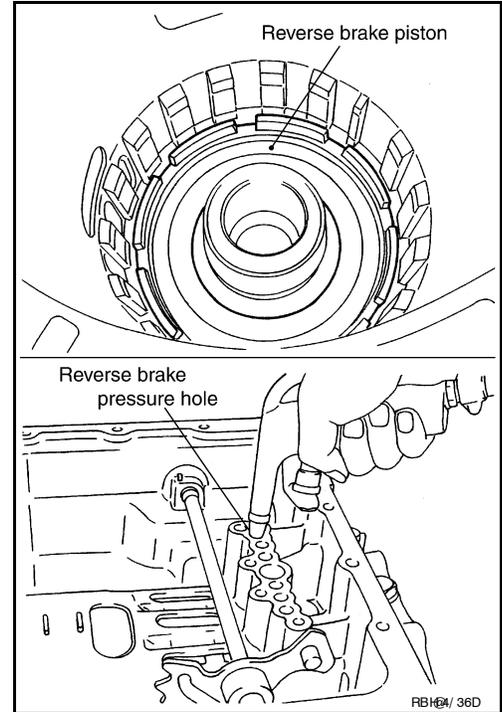
59. Remove D-rings from reverse brake piston.
