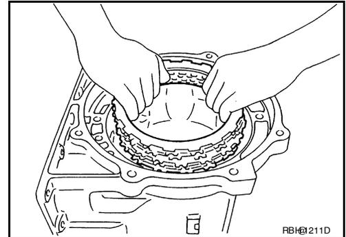
54. Remove snap ring using suitable tool.
