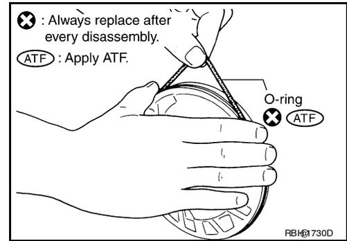
4. Remove O-ring from oil pump cover.
