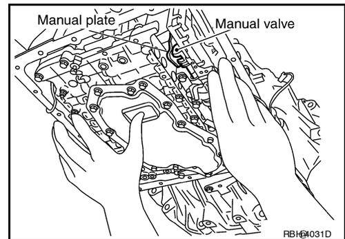
8. Install bolts (A), (B) and (C) in control valve with TCM. Tighten bolt (1), (2) and (3) temporarily to prevent dislocation. After that tighten them in order (1 → 2 → 3). Then tighten other bolts. Tighten control valve with TCM bolts to the specified torque.
