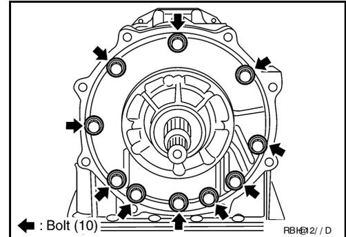
7. Remove the oil pump assembly evenly from the transmission case using Tools.
