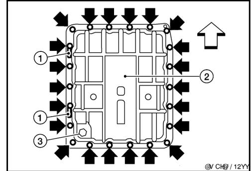
5. Check for foreign materials in oil pan to help determine cause of malfunction. If the A/T fluid is very dark, has some burned smell, or contains foreign particles then friction material (clutches, band) may need replacement. A tacky film that will not wipe clean indicates varnish build up. Varnish can cause valves, servo, and clutches to stick and can inhibit pump pressure.
