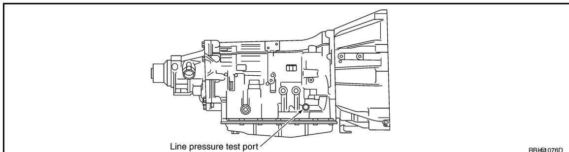
Line Pressure Test Procedure
