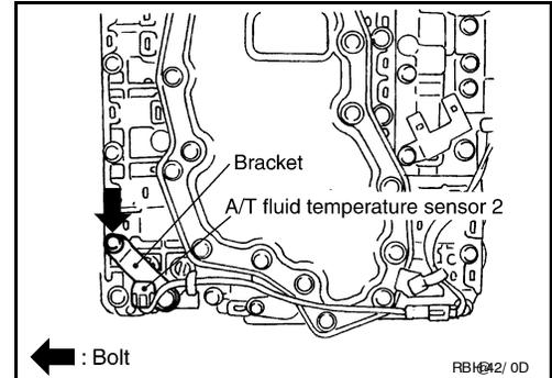
g. Install control valve with TCM in transmission case.
