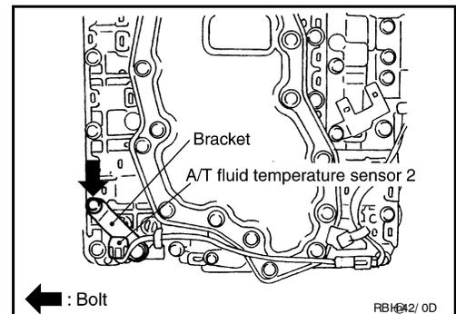
14. Remove bracket from A/T fluid temperature sensor 2.
