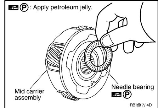
19. Remove needle bearing (rear side) from mid carrier assembly.
