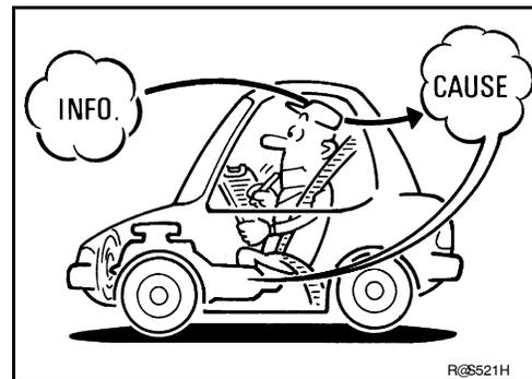
Before undertaking actual checks, take a few minutes to talk with a customer who approaches with a driveability complaint. The customer can supply good information about such errors, especially intermittent ones. Find out what symptoms are present and under what conditions they occur. A "Diagnostic work sheet" as shown on the example (Refer to [TM-76](#)) should be used.
