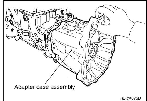
iii. Tighten adapter case assembly to specified torque.
