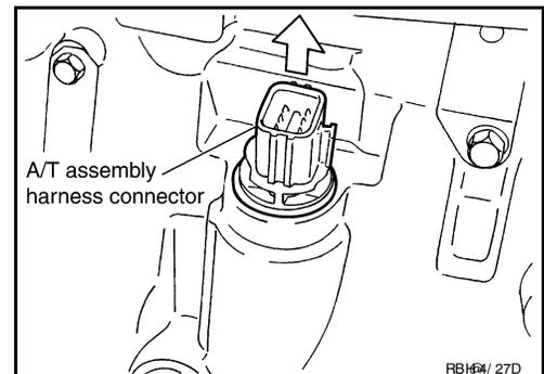
15. Install snap ring to A/T assembly harness connector.
