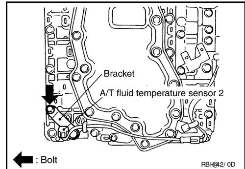
7. Install control valve with TCM in transmission case.
