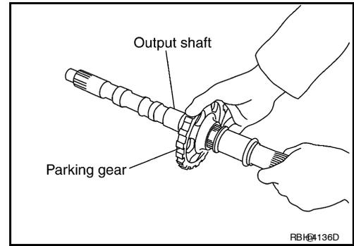
47. Remove seal rings from output shaft.
