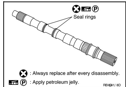
31. Install parking gear to output shaft.
