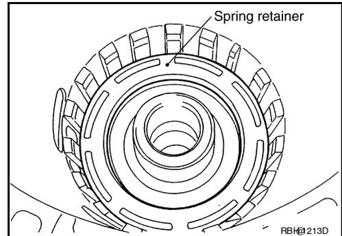
17. Install snap ring in transmission case while compressing return spring using Tool.
