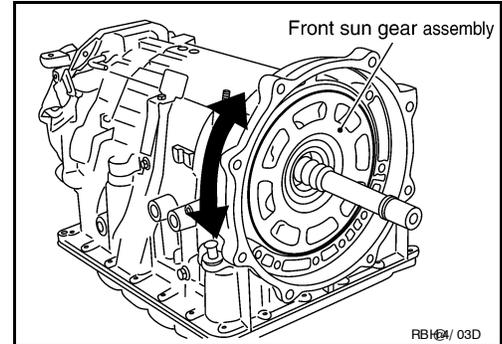
51. Install needle bearing to front sun gear.
