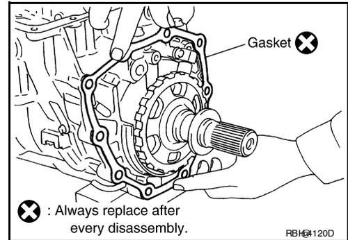
44. Remove bearing race from output shaft.
