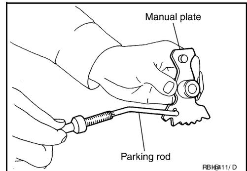
64. Remove manual shaft from transmission case.
