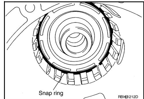
55. Remove spring retainer and return spring from transmission case.
