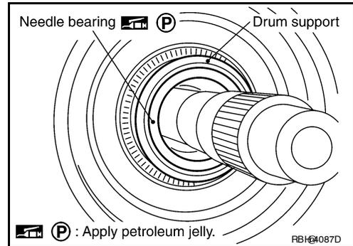
37. Install high and low reverse clutch assembly in direct clutch.
