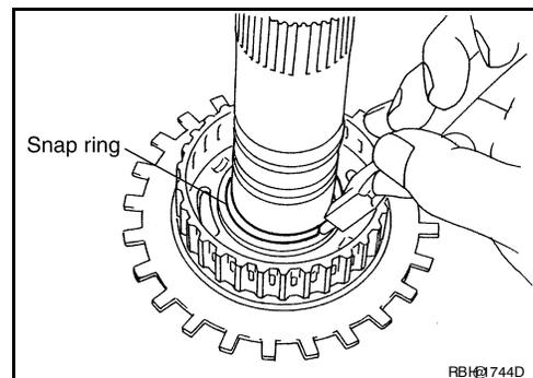
8. Check operation of 1st one-way clutch.
