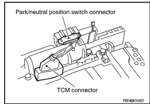
2. Install A/T assembly harness connector to control valve with TCM.
