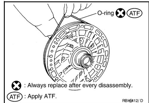
2. Install O-ring to oil pump housing.
