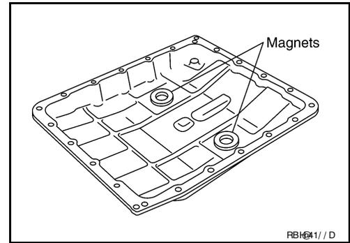
17. Install oil pan to transmission case. Refer to [TM-252. "Removal and Installation"](#).
