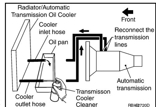
7. Tie a common white, basket-type coffee filter to the end of the cooler inlet hose.
