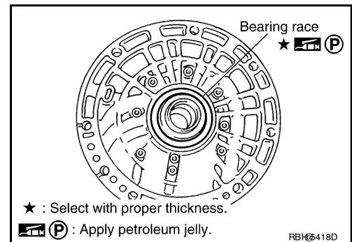
3. Install oil pump assembly in transmission case.
