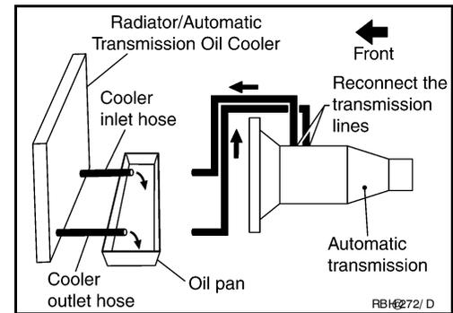
5. Insert the extension adapter hose of a can of Transmission Cooler Cleaner (Nissan P/N 999MP-AM006) into the cooler outlet hose.
