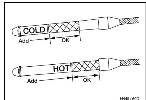
8. Install the A/T fluid level gauge in the A/T fluid charging pipe and install the A/T fluid level gauge bolt.
