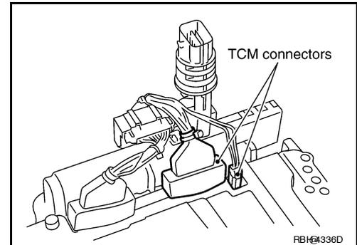
41. Remove A/T assembly harness connector from control valve with TCM using suitable tool.
