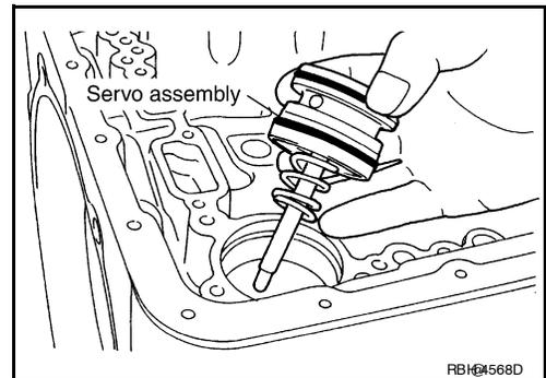
69. Remove return spring from servo assembly.
