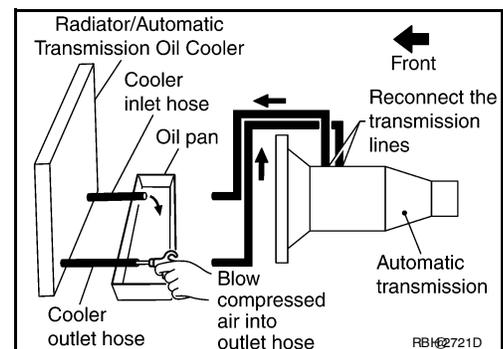
9. Blow compressed air regulated to 5 - 9 kg/cm<sup>2</sup> (71 - 128 psi) through the cooler outlet hose for 10 seconds to force out any remaining fluid.
