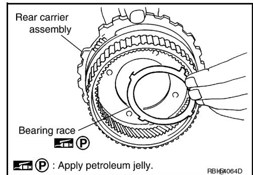
42. Install rear carrier assembly in direct clutch drum.
