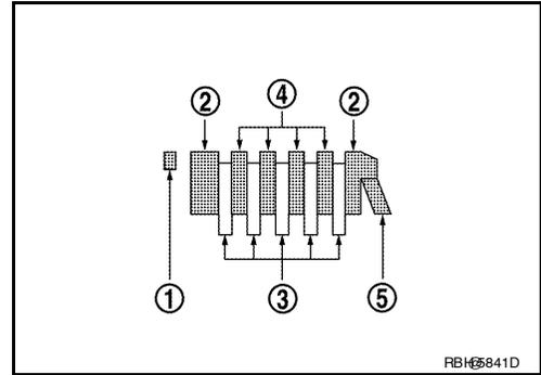
2. Install snap ring in direct clutch drum using suitable tool.
