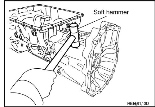
iii. Remove adapter case assembly (with needle bearing) from transmission case.
