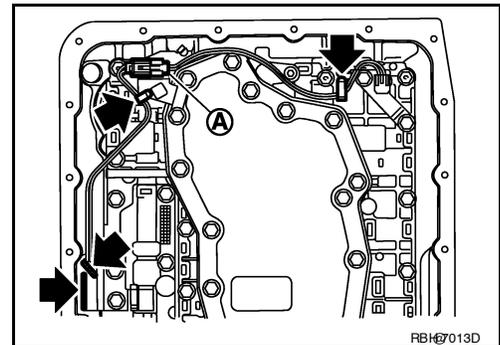
9. Straighten terminal clip to free the revolution sensor harness.
