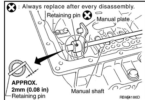
7. Install retaining pin into the transmission case and manual shaft.
