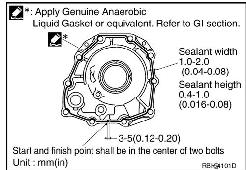
ii. Install rear extension assembly to transmission case.
