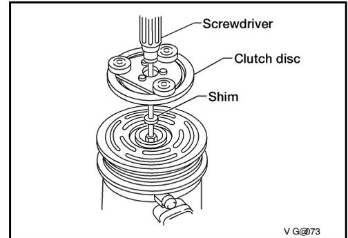
5. Install the clutch pulley bolt using Tool, to prevent the clutch disc from turning and tighten the bolt to specification. Refer to [HA-29, "Component"](#).
