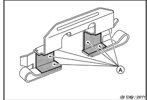
3. Attach pad retainer to torque member, then install brake pad and shim assemblies.
