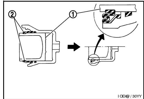
5. Apply rubber grease to the sliding pin boots, then install the sliding pins and sliding pin boots on the torque member.
