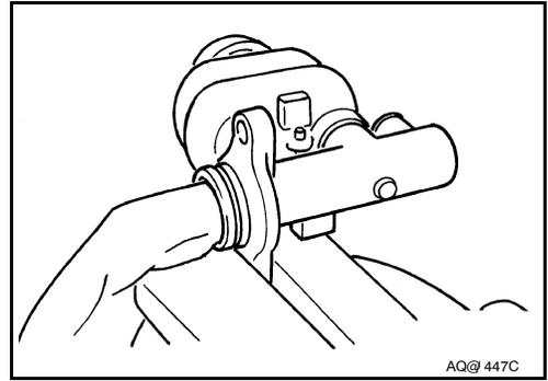
2. Remove the pin and pull the reservoir tank off of the master cylinder sub-assembly.
