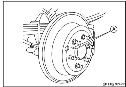
2. Install torque member and tighten the torque member bolts to specification. Refer to [BR-38. "Exploded View of Brake Caliper"](#).
