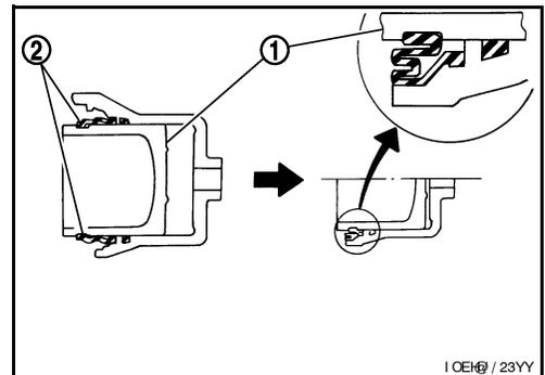
5. Apply rubber grease to the sliding pin boots, then install the new upper sliding pin, lower sliding pin, and sliding pin boots on the torque member.
