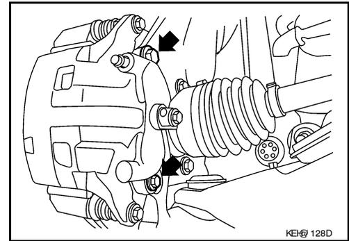
5. Remove the brake pads, shims, shim covers and retainers from the torque member.
