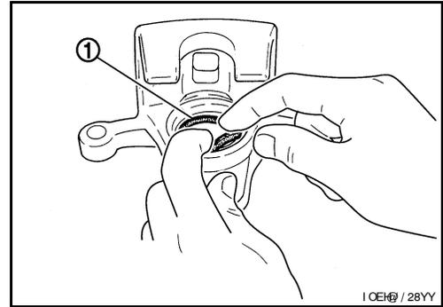
3. Apply rubber grease to the new piston boot (1). Cover the piston end (2) with the piston boot (1), and then install the cylinder side lip on the piston boot (1) securely into the groove on the cylinder body.
