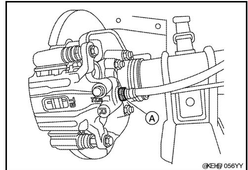
6. Refill with new brake fluid as necessary and bleed the air. Refer to [BR-17. "Bleeding Brake System"](#).
