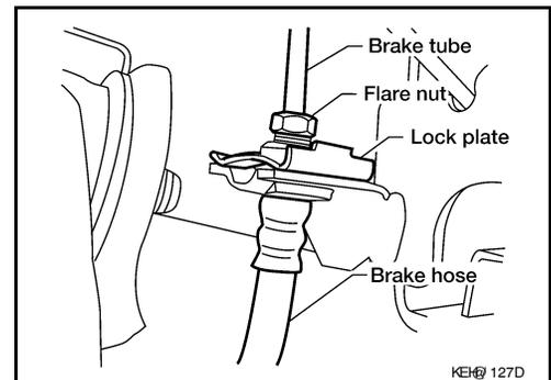
4. Refill brake fluid and bleed air. Refer to [BR-17, "Bleeding Brake System"](#).
