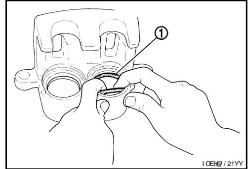
3. Apply rubber grease to the new piston boots (1). Cover the piston end (2) with the piston boot (1), and then install the cylinder side lip on the piston boot (1) securely into the groove on the cylinder body.
