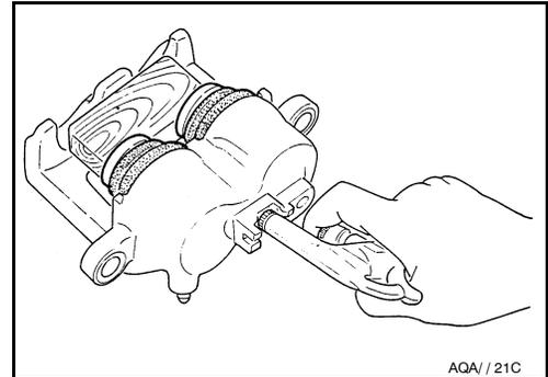
4. Remove the piston boots from the pistons.
