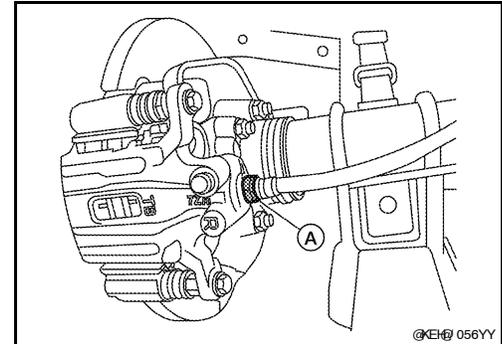
6. Remove the sliding pin bolts (A) and remove the caliper body from the torque member.
