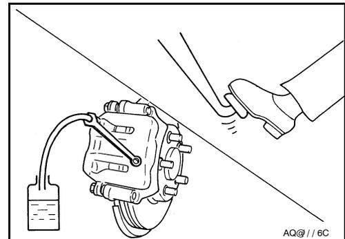
4. Make sure there is no foreign material in reservoir tank, and refill with new brake fluid.
