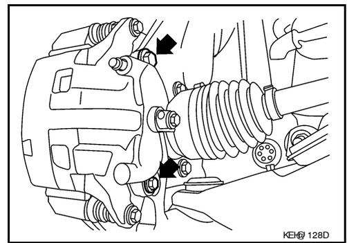
5. Install brake hose by aligning with the protrusion on caliper body, then install new copper washers and union bolt. Tighten union bolt to specified torque. Refer to [BR-33, "Exploded View of Brake Caliper"](#).
