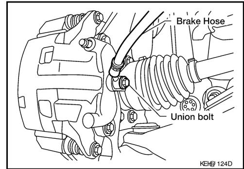
4. Remove the sliding pin bolts and remove the caliper body from the torque member.
