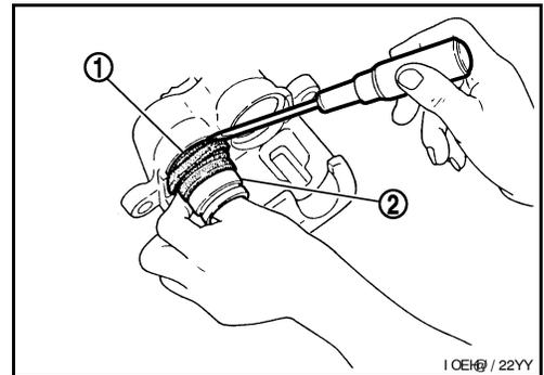
4. Install the pistons (1) into the cylinder body and insert the piston boots (2) side lip into the piston groove as shown.
