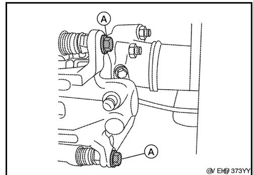
5. Connect the brake hose to the caliper body, using a new copper washer. Tighten the hose connection (A) to the specified torque. Refer to [BR-12. "Hydraulic Circuit"](#).
