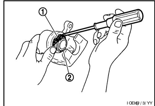
4. Install the piston (1) into the cylinder body and insert the piston boot (2) side lip into the piston groove as shown.
