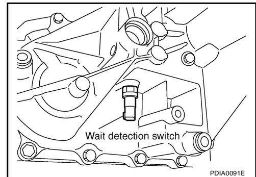
10. Remove check plug, check shift spring and check ball (M/T models only).
