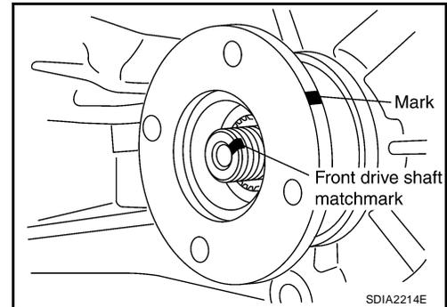
3. Install the new self-lock nut and tighten to the specified torque, using Tool. Refer to [TF-112, "COMPONENTS"](#).
