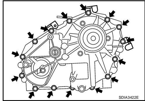
29. Install the retainer bolts with new gaskets. Tighten the bolts to the specified torque. Refer to [TF-112, "COMPONENTS"](#) .
