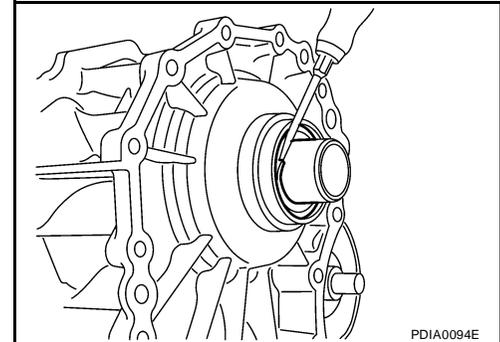
14. Remove the retainer bolts and gaskets.
