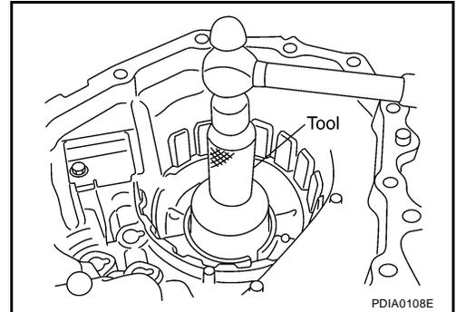
4. Install the new snap ring to the front case.
