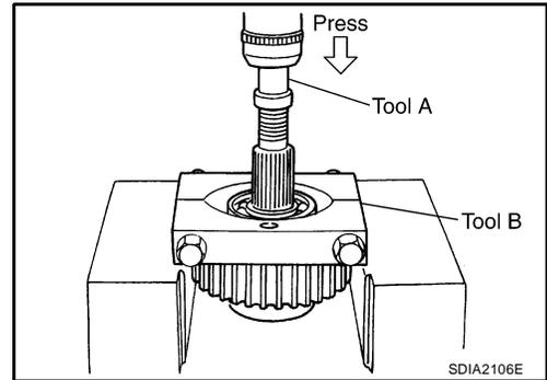
2. Remove the rear bearing, using Tools.
