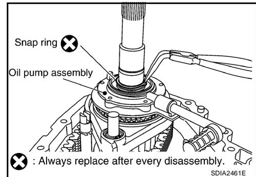
23. Remove the snap ring from the mainshaft, using suitable tool.
