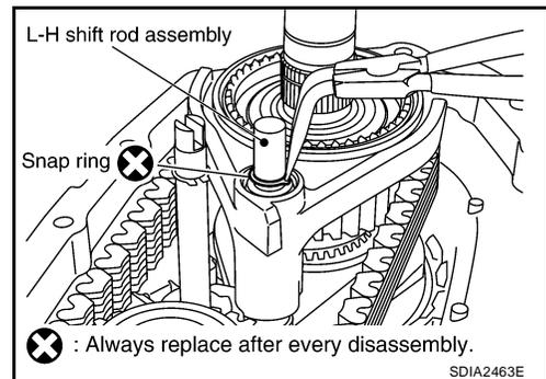
19. Install the new snap ring to the mainshaft, using suitable tool.
