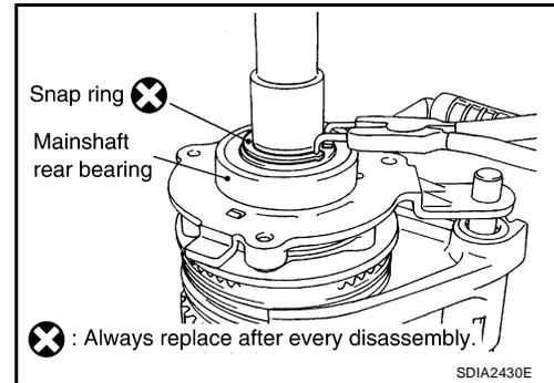
19. Remove the mainshaft rear bearing from the mainshaft, using suitable tool.
