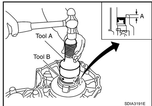
31. Install the new rear oil seal until it is flush with the end face of the rear case, using Tool.
