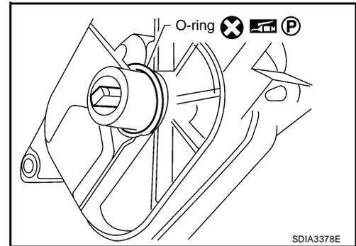
2. Install the transfer control device.
