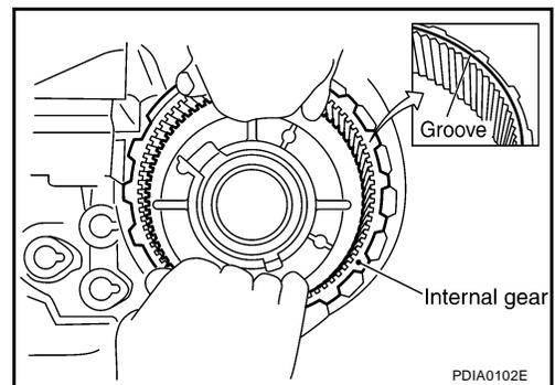
6. Install the new snap ring to the front case.
