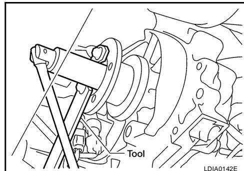
4. Put a matching mark on top of the front drive shaft in line with the mark on the companion flange.
