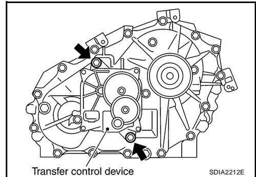
43. Install the drain plug and filler plug with new gaskets to the rear case. Tighten to the specified torque. Refer to [TF-112, "COMPONENTS"](#).
