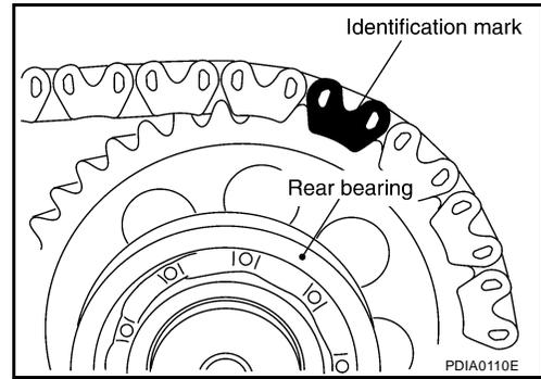
15. Install the drive chain together with the front drive shaft and sprocket to the front case.
