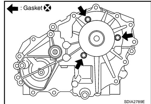
15. Remove the rear case bolts, harness bracket and air breather hose clamp from the rear case.
