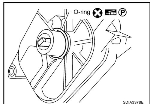
42. Install the transfer control device to the rear case.
