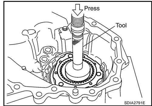
8. Install the new snap ring to the sun gear.
