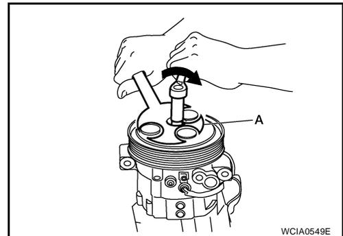
6. Check the pulley clearance all the way around the clutch disc as shown.
