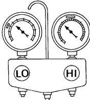
AC356A | High- and low-pressure sides become equal soon after A/C compressor operation stops. | A/C compressor pressure operation is improper.<br>↓<br>Damaged inside A/C compressor packings. | Replace A/C compressor. |
