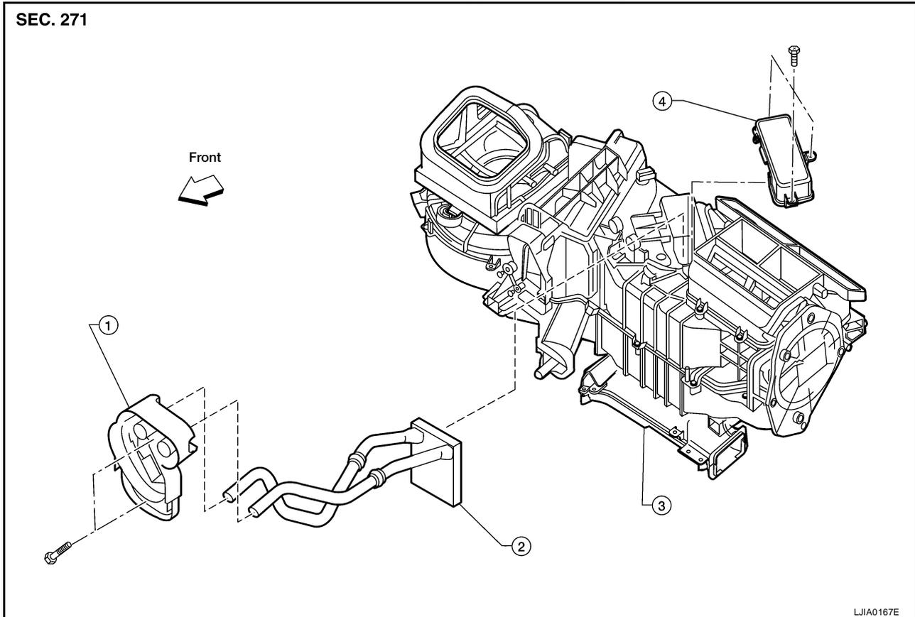
1. Heater core and evaporator pipe bracket
