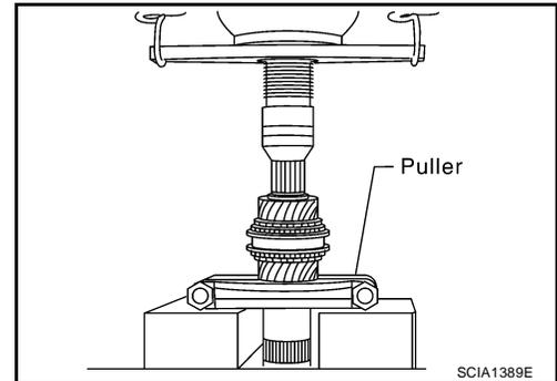
26. Press out 3rd gear bushing using suitable tool.
