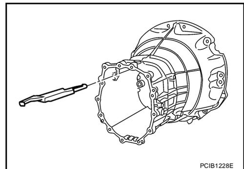
20. Remove filler plug and gasket from transmission case.
