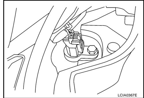
15. Tilt the transmission slightly to gain clearance between the body and the transmission, then disconnect the air breather hoses. Refer to [MT-16, "Removal and Installation"](#) .
