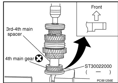
9. Press in mainshaft bearing using Tool.
