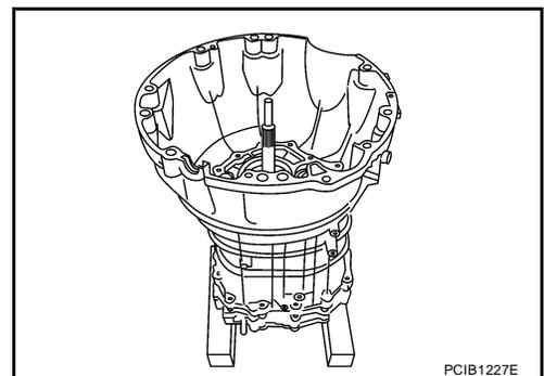
7. Install snap ring to main drive gear bearing using suitable tool.
