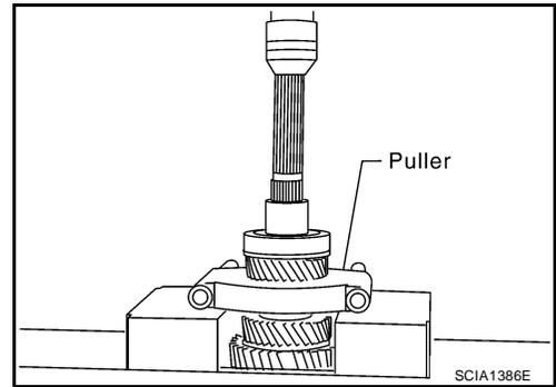
19. Remove 3rd main gear and 1st main gear according to the following.
