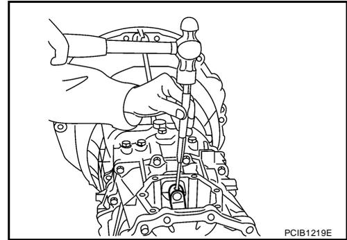
7. Remove rear extension (or OD gear case) bolts, and then remove rear extension (or OD gear case) from adapter plate using suitable tool.
