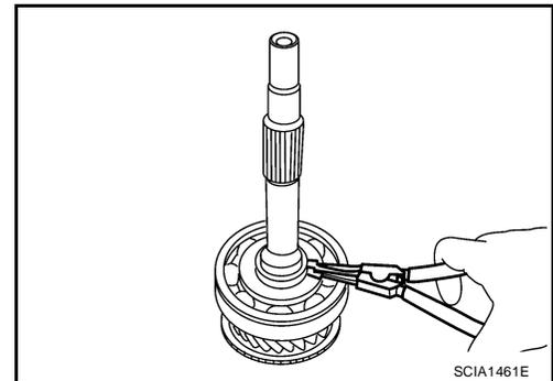
b. Press out main drive gear bearing using suitable tool.
