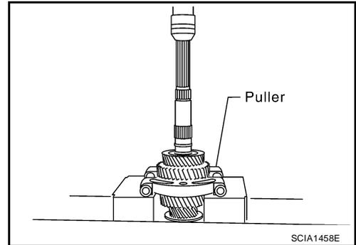
20. Remove 1st-2nd synchronizer hub assembly and 2nd main gear according to the following.
