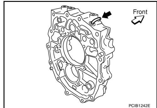
17. Install magnet to adapter plate.
