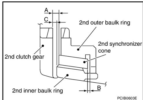
1. Measure the clearance "A" at 2 points or more diagonally opposite using a feeler gauge when pressing baulk ring toward clutch gear taper cone. Then calculate the mean value.
