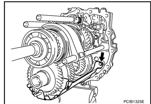
4. Remove check ball plugs, check ball springs and check balls from adapter plate.
