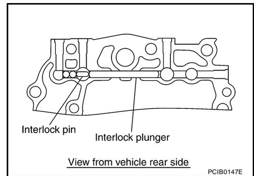
9. Install 1st-2nd fork rod according to the following.
