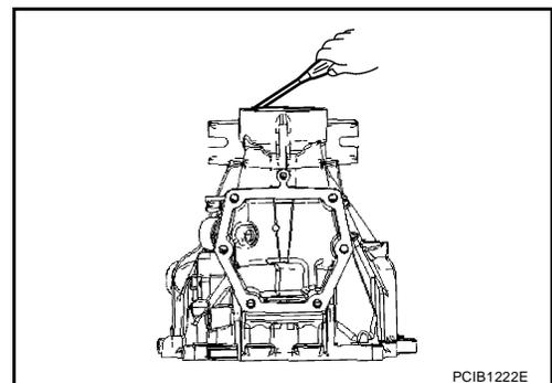
10. Remove counter end bearing from rear extension (or OD gear case) using suitable tool.
