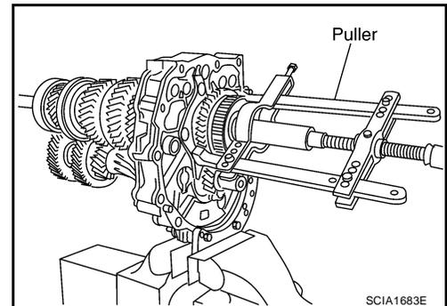
6. Remove reverse coupling sleeve according to the following.
