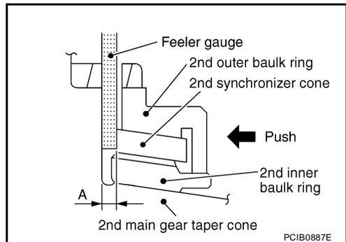
2. Measure the clearance "B" at 2 points or more diagonally opposite using a feeler gauge. Then calculate the mean value.
