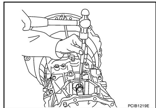
24. Install control housing according to the following.
