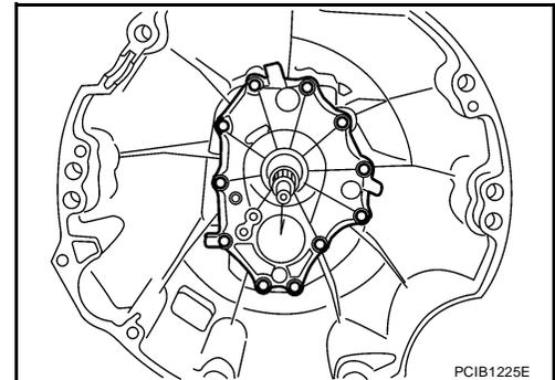
13. Remove front cover oil seal from front cover using suitable tool.
