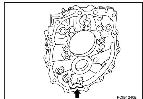
13. Remove baffle plate bolt, and then remove baffle plate from adapter plate.
