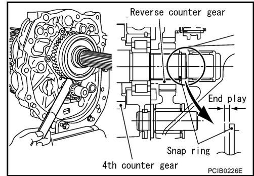
4. Remove reverse idler gear according to the following.
