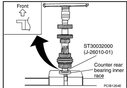
15. Install main drive gear bearing according to the following.
