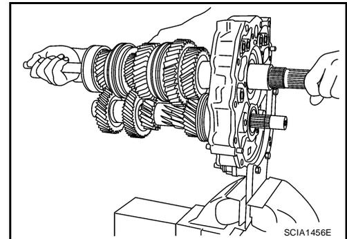
11. Remove counter rear bearing from adapter plate.
