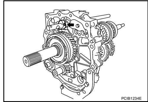
17. Remove striking rod assembly from adapter plate.
