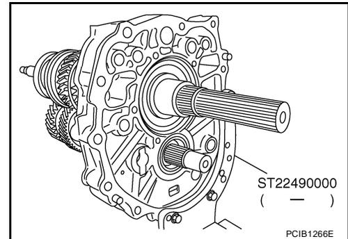
21. Install snap ring to mainshaft bearing.
