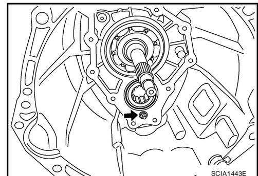
15. Remove snap ring from main drive gear bearing using suitable tool.
