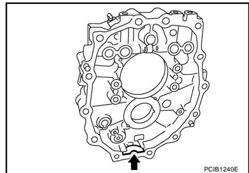
18. Install baffle plate to adapter plate, and then tighten bolt to the specified torque. Refer to [MT-22, "Case Components"](#).
