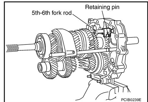
14. Remove 5th-6th control lever bolts, and then remove 5th-6th control lever from adapter plate.
