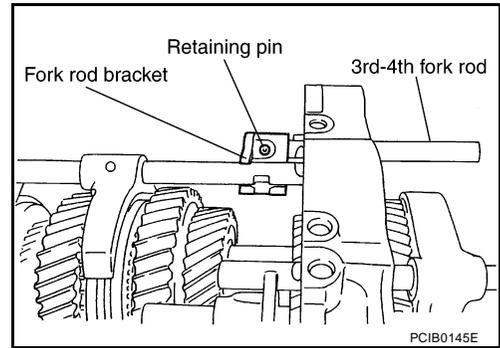
13. Install 3rd-4th control lever according to the following.
