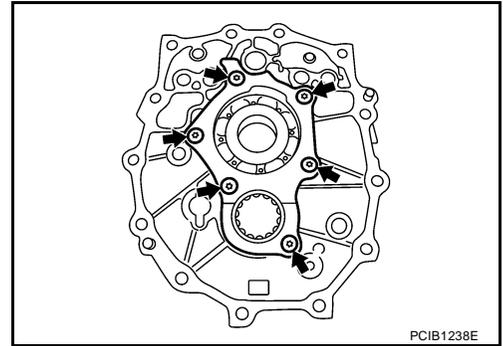
25. Install reverse synchronizer hub assembly according to the following.
