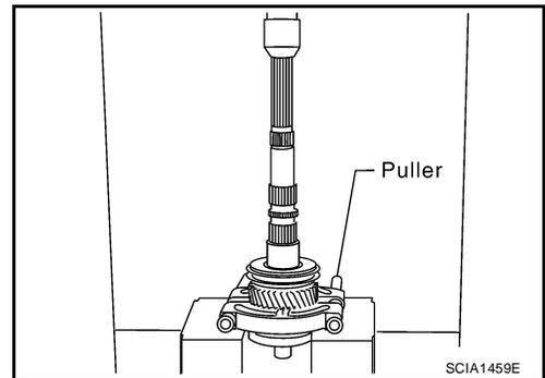
22. Remove 6th main gear and 5th-6th synchronizer hub assembly according to the following.
