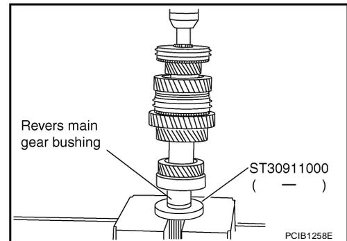
11. Press in 3rd gear bushing using Tool.
