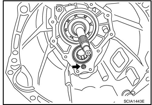
9. Tighten baffle plate bolt to the specified torque. Refer to [MT-22](#), "[Case Components](#)".
