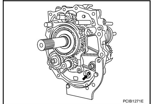
10. Install front cover oil seal to front cover using Tool.
