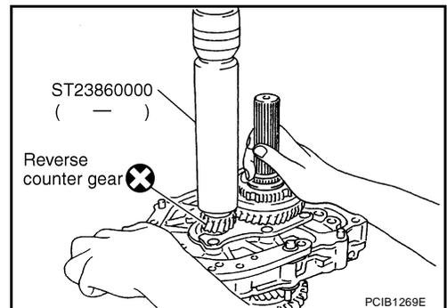
28. Select and install a snap ring so that the end play comes within the standard value. Refer to [MT-70, "Snap Rings"](#) .
