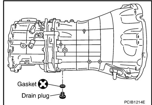
26. Install gasket to filler plug, and then install it to transmission case. Tighten filler plug to the specified torque. Refer to [MT-22, "Case Components"](#) .
