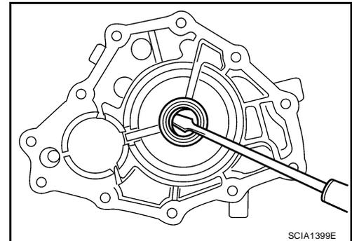
14. Remove baffle plate nut from transmission case.
