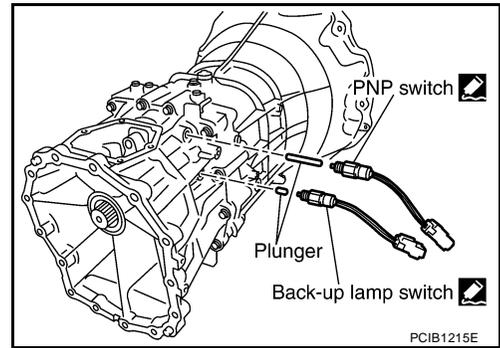
22. Install clips to PNP switch and back-up lamp switch.
