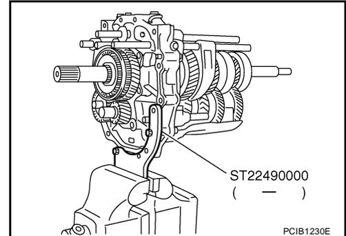
3. Remove baffle plate bolts, and then remove baffle plate from adapter plate.
