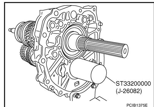
24. Install bearing retainer according to the following.
