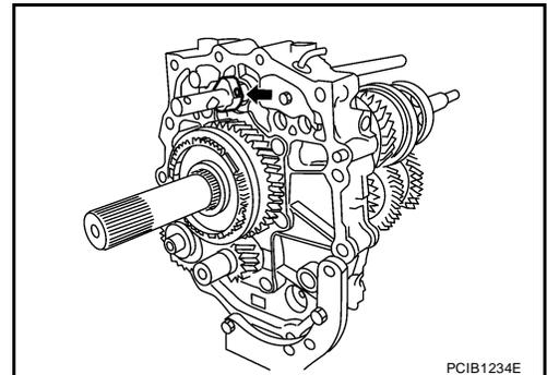
3. Install 5th-6th fork rod (reversal side) according to the following.
