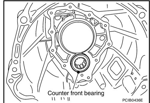
5. Apply recommended sealant to mating surface of transmission case as shown.
