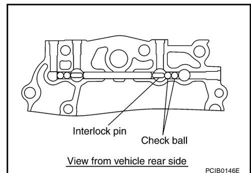
11. Install 3rd-4th fork rod (reversal side) according to the following.
