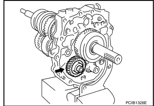
5. Remove reverse main gear and reverse synchronizer hub assembly according to the following.
