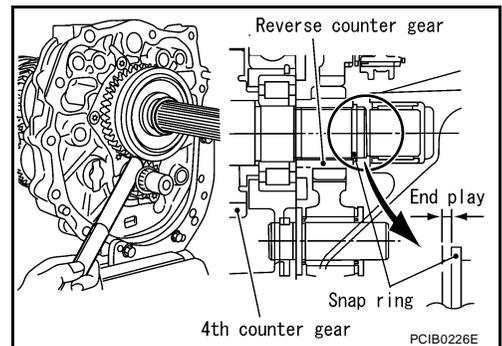
29. Install reverse idler shaft assembly according to the following.
