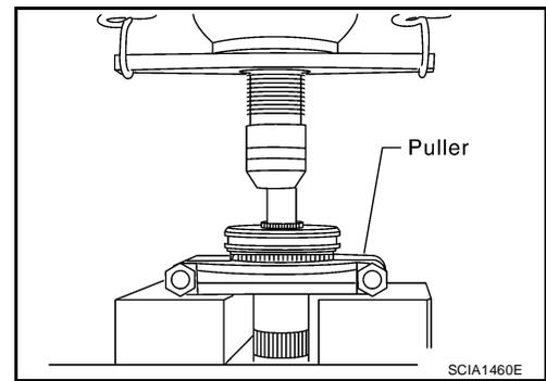
24. Remove 3rd counter gear, 3rd-4th synchronizer hub assembly, 4th counter gear according to the following.
