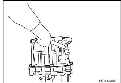
8. Remove rear extension oil gutter bolt, and then remove rear extension oil gutter and cap from rear extension. (For 2WD models)
