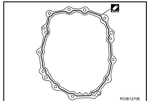
6. Install transmission case to adapter plate assembly.
