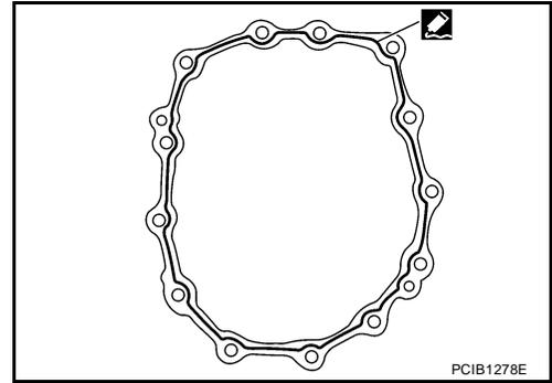
18. Install rear extension (or OD gear case) to adapter plate, and then tighten bolts to the specified torque in order as shown. Refer to [MT-22, "Case Components"](#).
