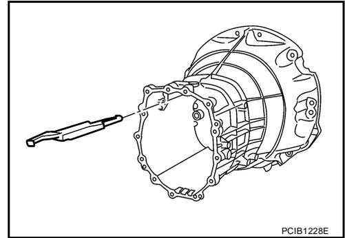
4. Install counter front bearing to transmission case.
