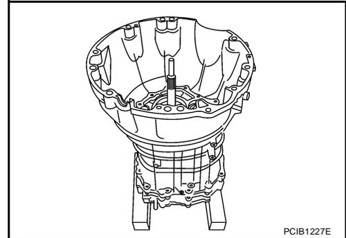
18. Remove counter front bearing from transmission case.
