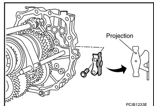
15. Remove retaining pin using suitable tool, and then remove 5th-6th shift fork and 5th-6th fork rod (reversal side) from adapter plate.
