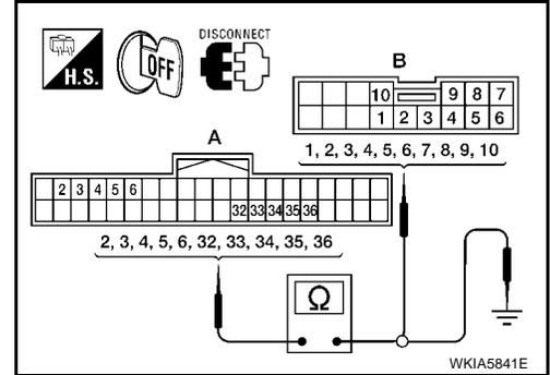
4. Check for continuity between each terminal of BCM harness connector in suspect malfunctioning system and ground.
