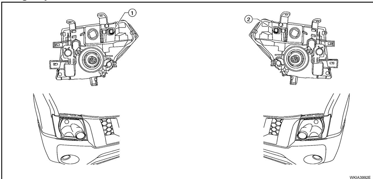
1. Adjustment screw (passenger side) 2. Adjustment screw (driver side)
