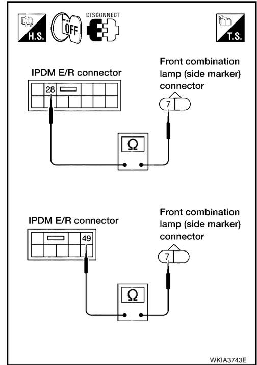
4. Check continuity between IPDM E/R harness connector and front combination lamp (parking) harness connector.
