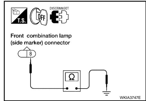
3. Check continuity between front combination lamp (parking) harness connector and ground.
