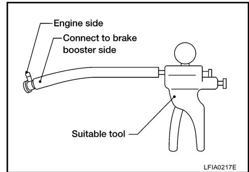
**Check valve specification** : Vacuum decrease should be within 1.3 kPa (10 mmHg, 0.39 inHg) for 15 seconds under a vacuum of – 66.7 kPa (– 500 mmHg, – 19.69 inHg)
