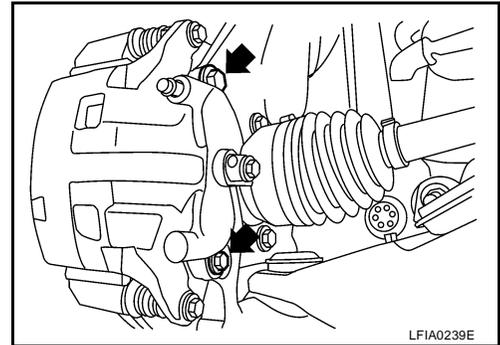
5. Install brake hose to cylinder body, if removed, then tighten union bolt to the specified torque. Refer to [BR-22, "Components"](#) .
