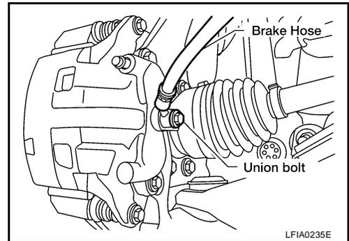
6. Refill new brake fluid and bleed air. Refer to [BR-10, "Bleeding Brake System"](#) .
