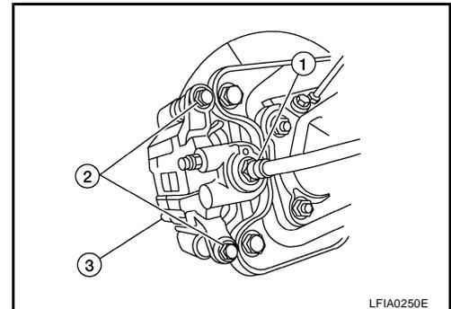
2. Insert brake hose end through bracket, then secure it to bracket with lock plate.
