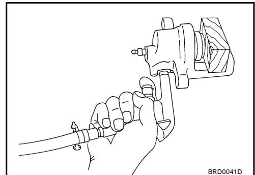
4. Remove piston seal from cylinder body using suitable tool.
