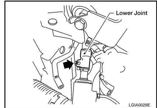
11. Remove the nuts and bolts of the steering gear assembly, using power tool, then remove the steering gear assembly from the vehicle.
