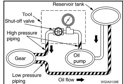
2. Start the engine. Run the engine until the power steering fluid temperature reaches 50 – 80°C (122 – 176°F).
