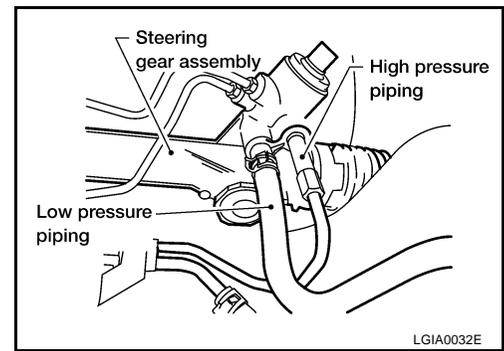
10. Remove the bolt from the lower joint of the lower joint shaft, then separate the lower joint from the steering gear assembly.
