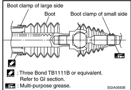
4. Install the boot clamps to the boots, as shown.
