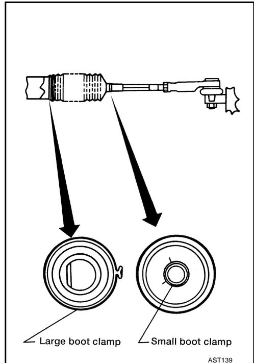
5. Crimp the large-diameter boot clamps, using Tool.
