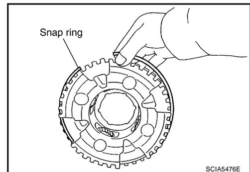
4. Disassemble input clutch assembly.
