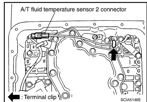
6. Remove A/T fluid temperature sensor 2 with bracket from control valve with TCM.
