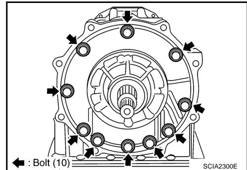
7. Attach the Tool to oil pump assembly and extract it evenly from transmission case.
