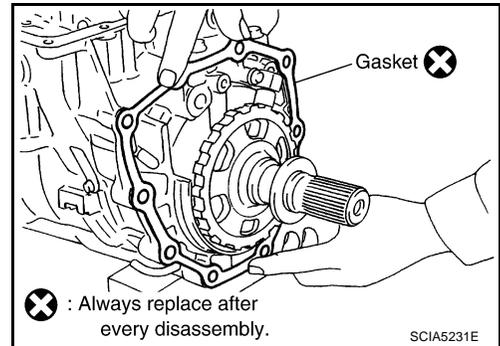
44. Remove bearing race from output shaft.
