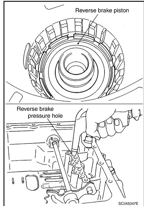
59. Remove D-rings from reverse brake piston.
