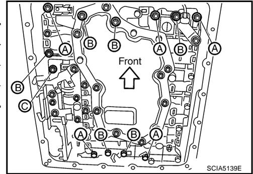
12. Remove control valve with TCM from transmission case.
