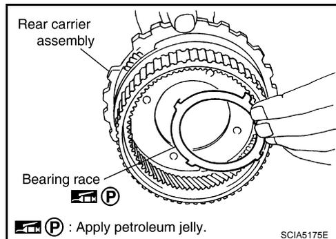
41. Install rear carrier assembly in direct clutch drum.
