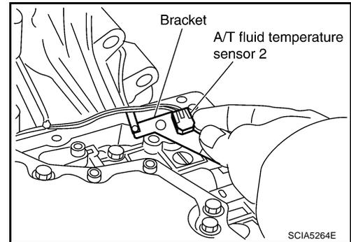
6. Install A/T fluid temperature sensor 2 (with bracket) in control valve with TCM. Tighten A/T fluid temperature sensor 2 bolt to the specified torque. Refer to [AT-234, "COMPONENTS"](#).
