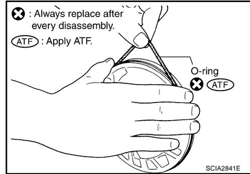
4. Remove O-ring from oil pump cover.
