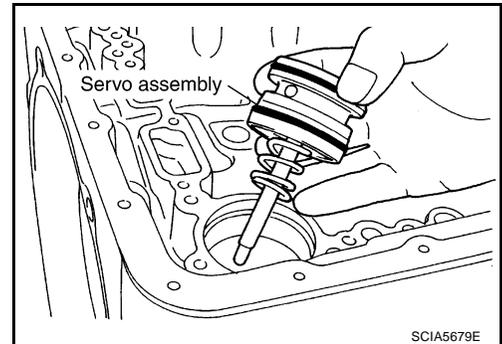
69. Remove return spring from servo assembly.
