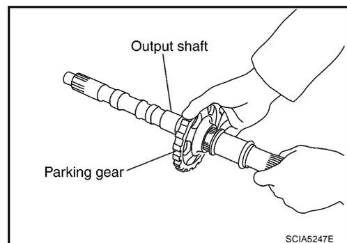
31. Install output shaft in transmission case.
