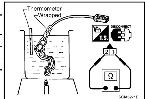
3. If NG, replace the A/T fluid temperature sensor 2. Refer to [AT-241, "A/T FLUID TEMPERATURE SENSOR 2 REMOVAL AND INSTALLATION"](#).
