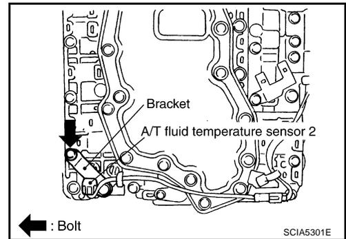
38. Remove bracket from A/T fluid temperature sensor 2.
