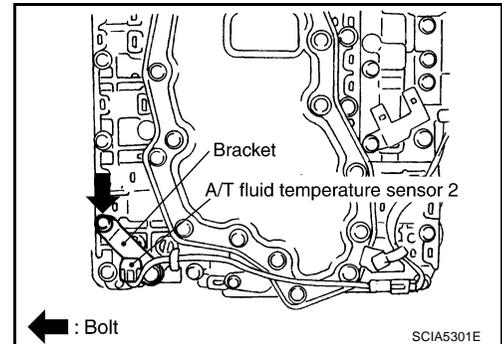
7. Install control valve with TCM in transmission case.
