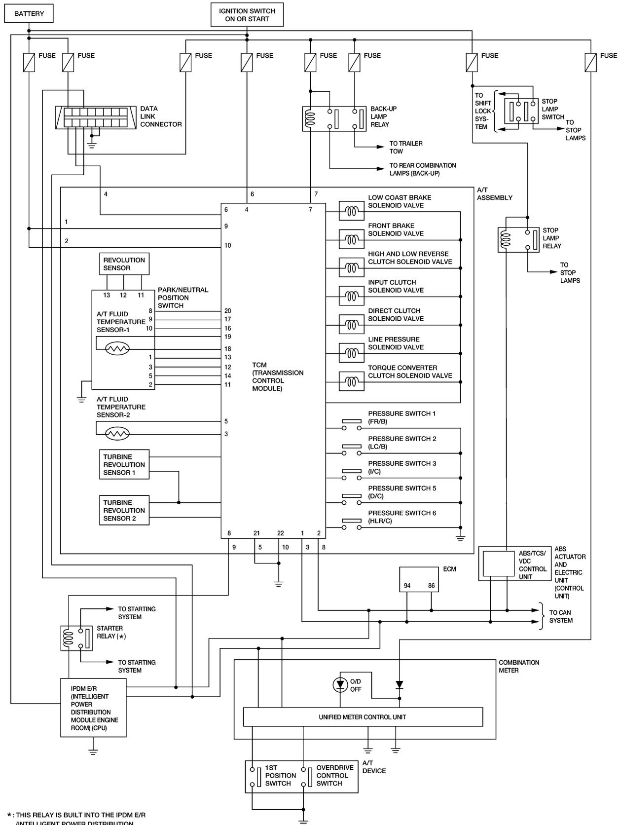
\*: THIS RELAY IS BUILT INTO THE IPDM E/R (INTELLIGENT POWER DISTRIBUTION MODULE ENGINE ROOM) (CPU)
