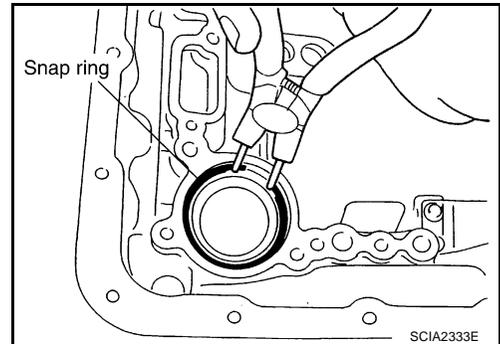
12. Install new D-rings in reverse brake piston.
