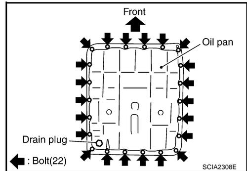
c. Tighten oil pan bolts to the specified torque in numerical order shown after temporarily tightening them.
