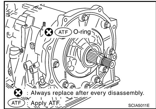
6. Remove bolts for oil pump assembly and transmission case.
