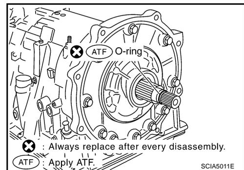
7. Install converter housing to transmission case.
