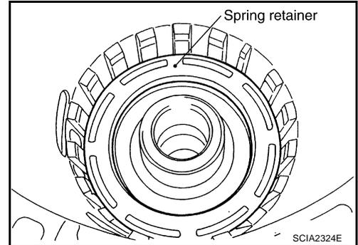
17. Install snap ring (fixing spring retainer) in transmission case while compressing return spring using Tool.
