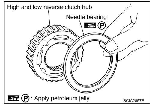
6. Install high and low reverse clutch hub to mid sun gear assembly.
