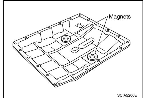
17. Install oil pan to transmission case.
