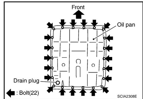
29. Check foreign materials in oil pan to help determine causes of malfunction. If the A/T fluid is very dark, smells burned, or contains foreign particles, the frictional material (clutches, band) may need replacement. A tacky film that will not wipe clean indicates varnish build up. Varnish can cause valves, servo, and clutches to stick and can inhibit pump pressure.
