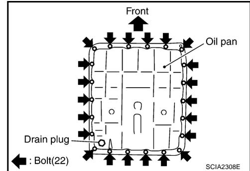
3. Check for foreign materials in oil pan to help determine cause of malfunction. If the A/T fluid is very dark, has some burned smell, or contains foreign particles then friction material (clutches, band) may need replacement. A tacky film that will not wipe clean indicates varnish build up. Varnish can cause valves, servo, and clutches to stick and can inhibit pump pressure.
