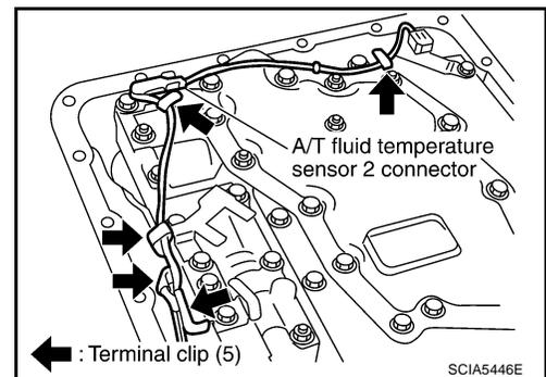
9. Straighten terminal clips to free revolution sensor harness.
