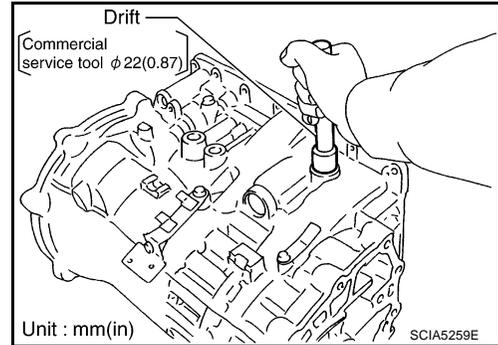
2. Install detent spring and spacer in transmission case.
