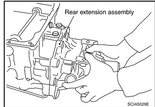
iii. Tighten rear extension assembly bolts to specified torque.
