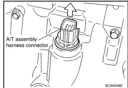
17. Install snap ring to A/T assembly harness connector.
