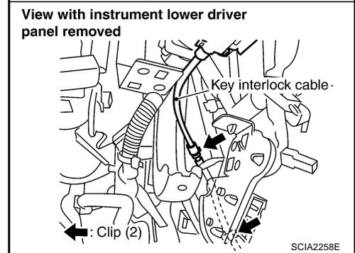
4. Insert interlock rod into adjuster holder.
