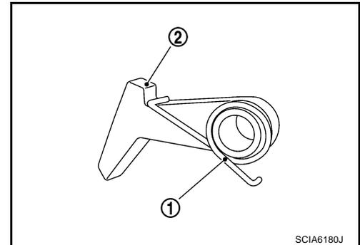
26. Install parking pawl (with return spring) and pawl shaft to rear extension (2WD models) or adapter case (4WD models).
