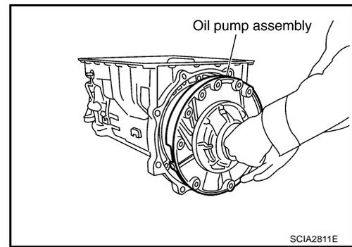
4. Apply recommended sealant (Genuine RTV Silicone Sealant or equivalent. Refer to [GI-46, "Recommended Chemical Products and Sealants"](#) .) to oil pump assembly as shown.
