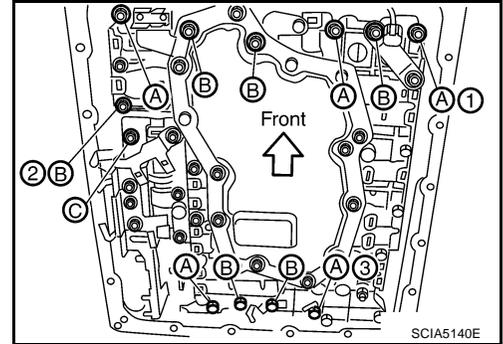
11. Connect A/T fluid temperature sensor 2 connector.
