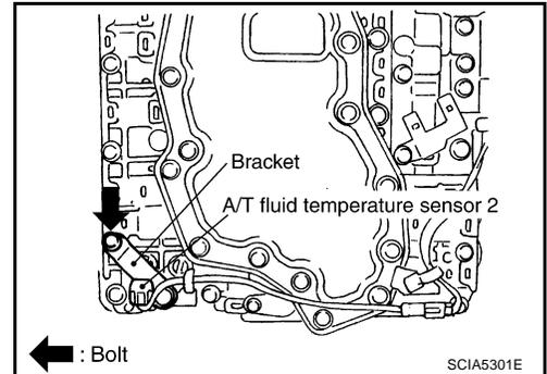
14. Remove bracket from A/T fluid temperature sensor 2.
