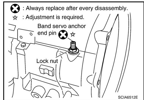
48. Install brake band in transmission case.
