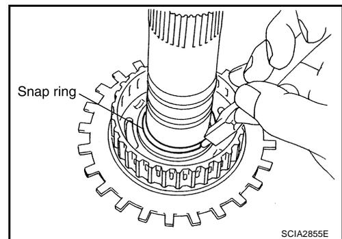
8. Check operation of 1st one-way clutch.
