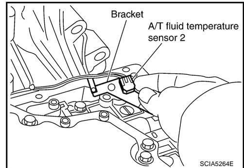
2. Install A/T fluid temperature sensor 2 (with bracket) in control valve with TCM. Tighten A/T fluid temperature sensor 2 bolt to the specified torque. Refer to [AT-234, "COMPONENTS"](#).
