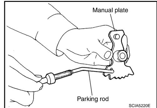
64. Remove manual shaft from transmission case.
