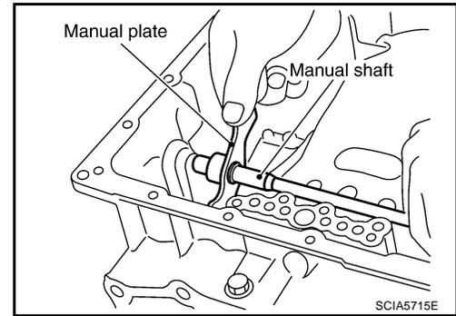
6. Install new retaining pin into the manual plate and manual shaft.
