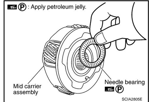
44. Install mid carrier assembly in rear carrier assembly.
