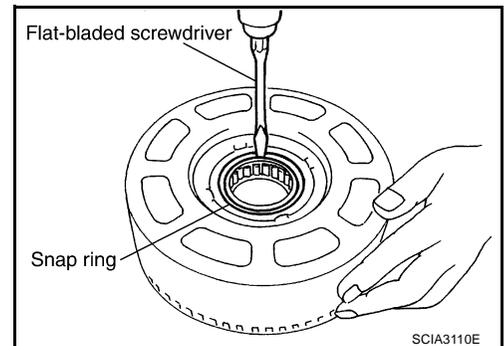
2. Remove 3rd one-way clutch from front sun gear.
