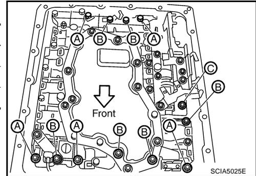
i. Tighten bolt 1, 2 and 3 temporarily to prevent dislocation. After that tighten them in order (1 → 2 → 3), and then tighten other bolts.
