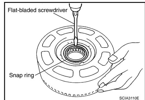
3. Check operation of 3rd one-way clutch.
