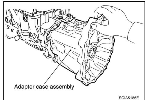
iii. Tighten adapter case assembly bolts (1) to specified torque. (With terminal bracket (2).)
