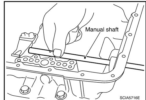
65. Remove manual shaft oil seals using suitable tool.
