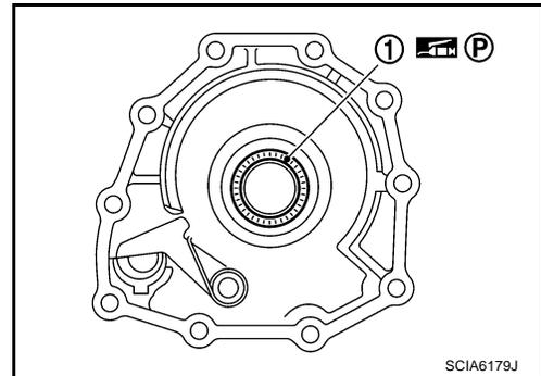
29. Install new seal rings to output shaft.
