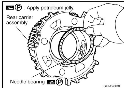
40. Install bearing race in rear carrier assembly.
