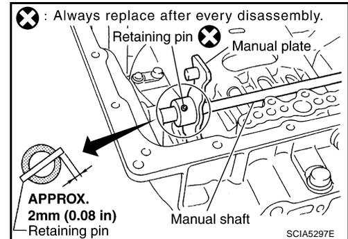
7. Install new retaining pin into the transmission case and manual shaft.
