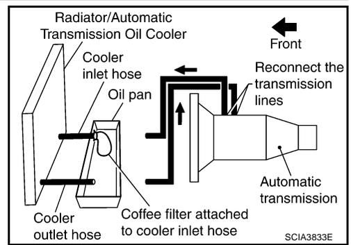
8. Insert the tip of an air gun into the end of the cooler outlet hose.
