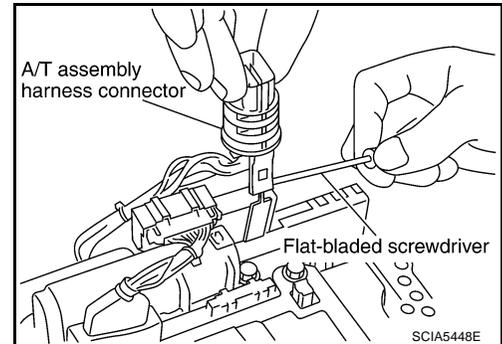
18. Disconnect TCM connector and park/neutral position switch connector
