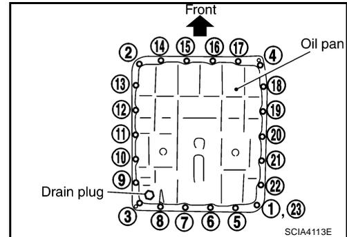
4. Install drain plug to oil pan.
