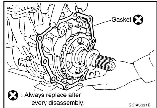
ii. Install adapter case assembly to transmission case.
