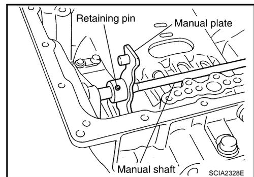
61. Remove manual shaft retaining pin using suitable tool.
