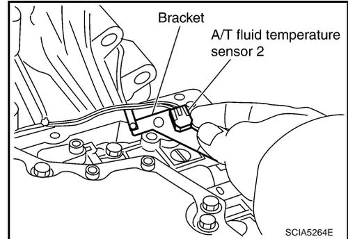
f. Install A/T fluid temperature sensor 2 (with bracket) in control valve with TCM.
