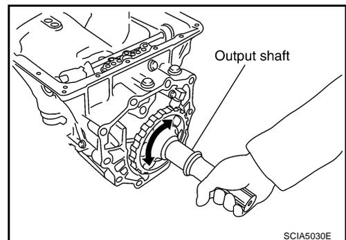
46. Remove parking gear from output shaft.
